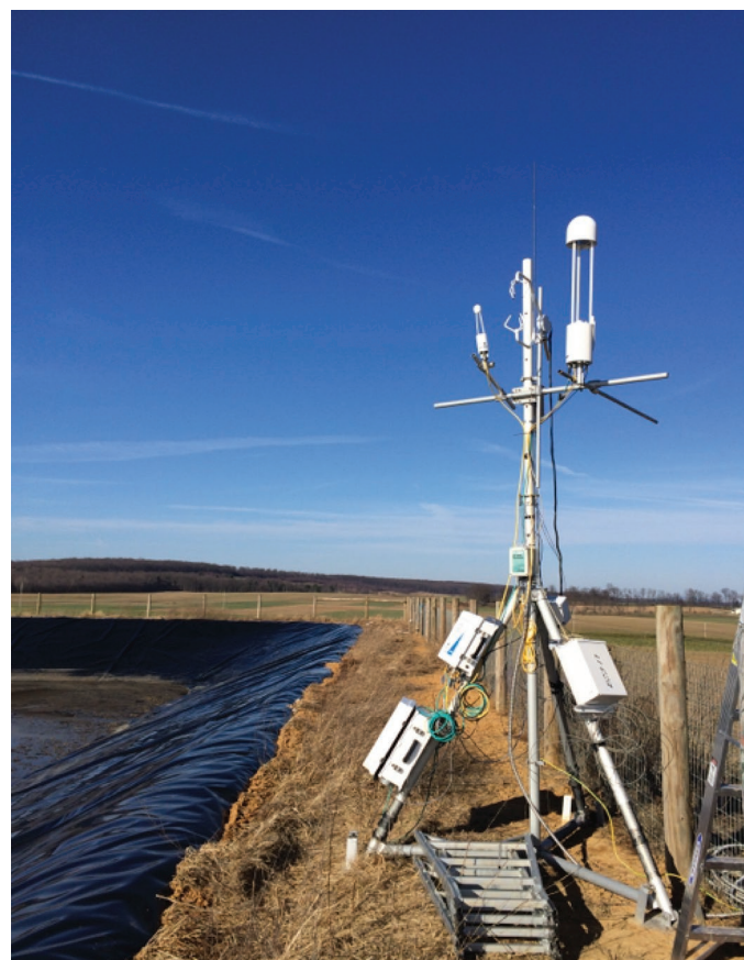
Figure 6. Manure emission measurement at a commercial dairy farm using the Eddy covariance technique (provided by A. N. Hristov, The Pennsylvania State University).
