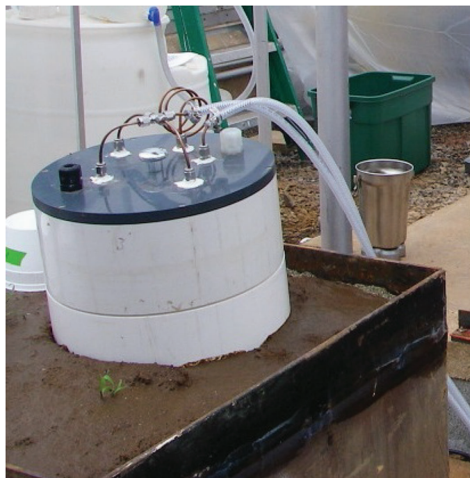
Figure 5. Measurement of ammonia emissions from the surface of manure-amended soil using a vented chamber (Lee et al., 2014; photo provided by A. N. Hristov, The Pennsylvania State University).
