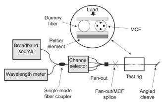
Fig. 5. Interrogation system with selectable addressing of the four MCF cores.
