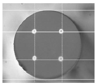
Fig. 1. MCF cross section. The core spacing is  $50 \mu m$ .
