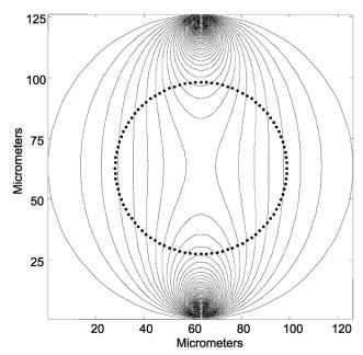
Fig. 10. Theoretical stress pattern of the MCF compressed by two diametrically opposite flat plates. The dotted circle shows the loci of points at which the cores sample the stress field.
