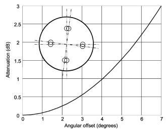
Fig. 2. Calculated attenuation due to angular misalignment between two MCFs.
