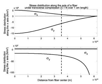
Fig. 11. Throughout the fiber cross section the horizontal normal stress  $\sigma_x$  is always positive or tensile and the vertical normal stress  $\sigma_y$  is negative or compressive. The dashed vertical lines indicate the radial location of the cores.
