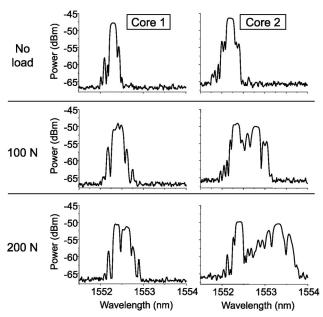
Fig. 4. Reflected FBG spectra from two MCF cores showing peak splitting under an increasing transverse load.
