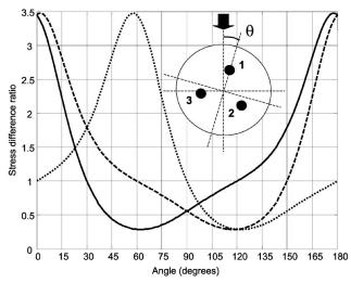
Fig. 13. Stress difference ratio simulated for the core pairs 1 and 2 (solid curve), 1 and 3 (dashed curve), 2 and 3 (dotted curve).
