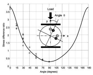
Fig. 8. Theoretical curve (solid curve) and experimental data (points) for the stress difference ratio of two cores at  $90^{\circ}$  separation.
