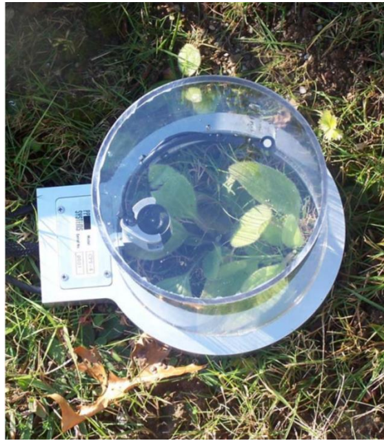
Figure 2: The CPY-4 transparent chamber used to measure efflux from low lying vegetation.
