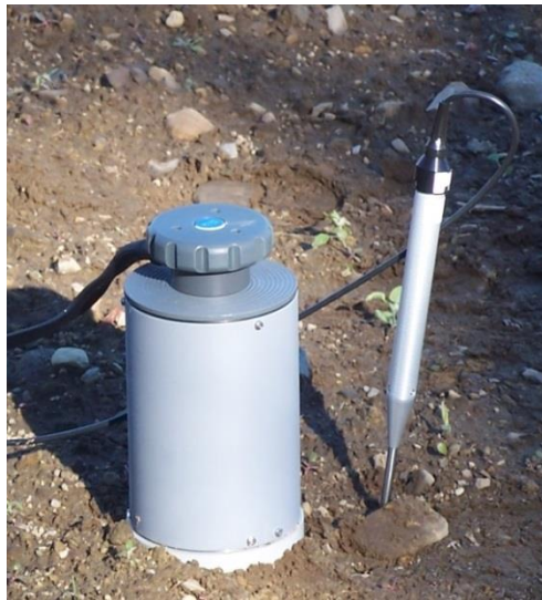
Figure 1: The PP Systems SRC-1 none transparent chamber model used to measure soil efflux.
