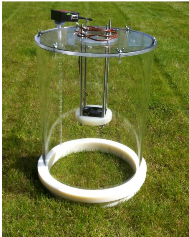
Figure 4: The used designed chamber at the University of the West of Scotland, located on the grass land site.
