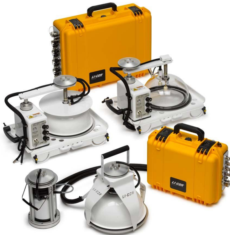
Figure 10: LI-8100A Automated Soil CO 2 Flux System and soil chambers provided by LICOR [79] .
