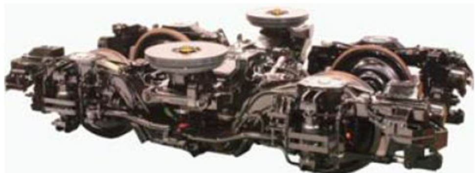
Fig. 3 Hybrid tilting bogie [7]
