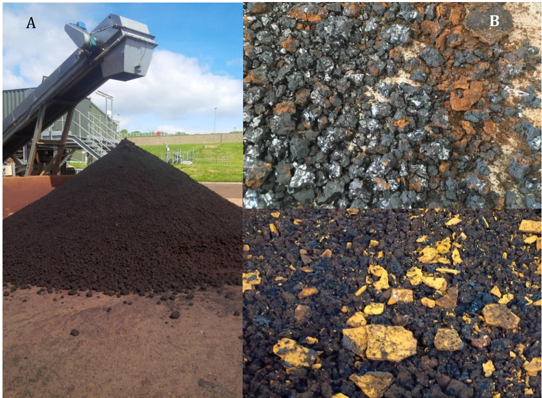
Figure 14: Photos of WTR, (a) freshly produced from the water treatment plant at Mosswood water treatment plant (b) oven-dried water treatment residual, clearly showing iron oxide (orange rust colour) precipitates.
