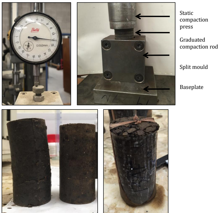
Figure 24: Split mould and static compaction press method. (a) Top left - Pressure gauge on static compaction press. (b) Top right - Split mould and static compaction press. (c) Bottom left - Samples with high compost additions (where left has been removed from mould immediately after compaction and right after 1 hour of pressure equilibration). (d) Bottom right - Finished sample with latex coating and geotextile wrap
