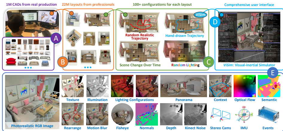
Figure 2: System Overview: an end-to-end pipeline to render an RGB-D-inertial benchmark for large scale interior scene understanding and mapping. (A) We collect around 1 million CAD furniture models from world-leading furniture manufacturers. These models have been used in the real-world production. (B) Based on those models, around 1,100 professional designers/companies create around 22 million interior layouts. Most of such layouts have been used in real-world decorations. (C) For each layout, we generate a number of configurations to represent different lightings and simulate scene change over time in daily life. (D) We provide an interactive simulator ( ViSim ) to create the ground truth monocular/stereo trajectories, as well as IMU and event camera data. Trajectories can be set manually, or using random walk and neural network based generation. (E) All supported image sequences and ground truth data.
