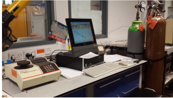
Fig. 8. The test set-up for determining true density.
