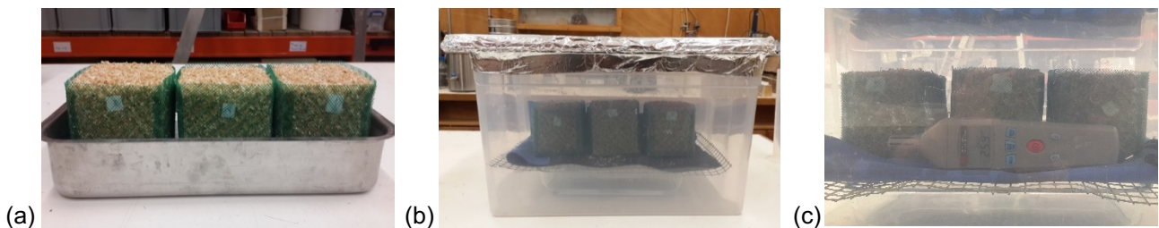
Fig. 6. a) The samples, b) The test set-up for desiccator method, c) The humidity / temperature meter inside the container.
