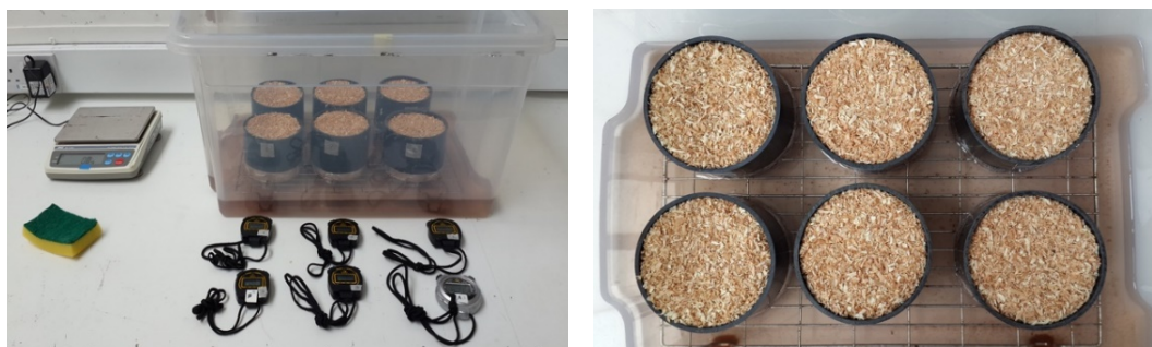
Fig. 10. The test set-up for the water absorption test.
