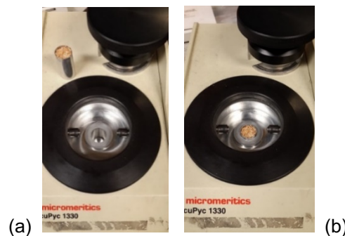
Fig. 9. a) The cup including WW b) The cup inserted into the cell chamber.
