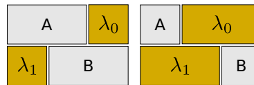
Figure 18. Two concrete layouts with the same layout specification s = (A|\lambda_0)/(\lambda_1|B) . On the left, areas A and B have a relatively large intrinsic preferred width. On the right, their preferred widths are relatively small.
