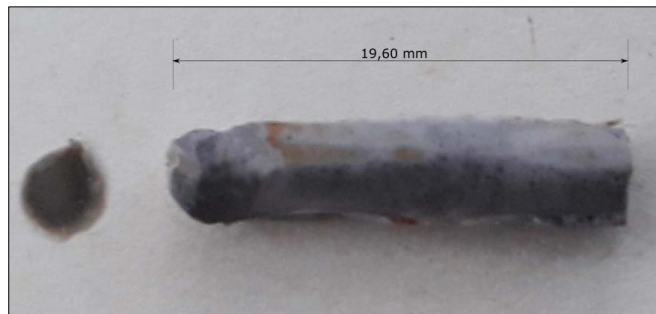
Figure 154: After the 5 h falling sphere experiment, an image of 1550 ppm CO 2 chlorine-bearing basalt with a crystallised surface.
