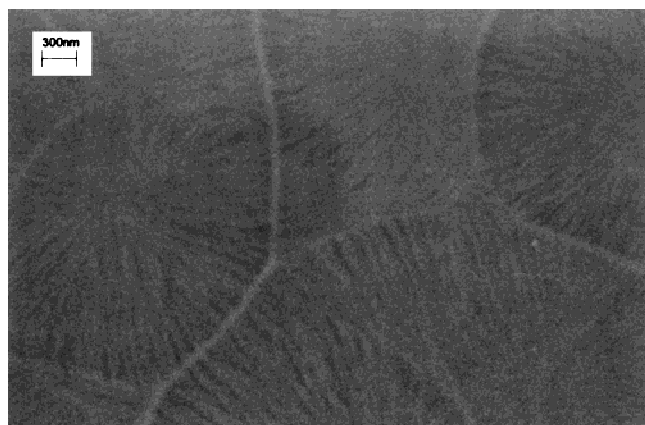
FIG. 1. Surface morphology of a type-A sample with a current density of 25 \text{ mA/cm}^2 and an etching time of 5 min.
