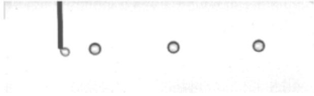
Figure 3-1. The drop generation process of V_c = 210.42 mm/s, and V_d = 543.67 mm/s.
