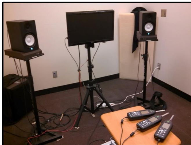
Figure 53: Perceptual Test Item Creation – Audio File Acoustical Verification Setup
