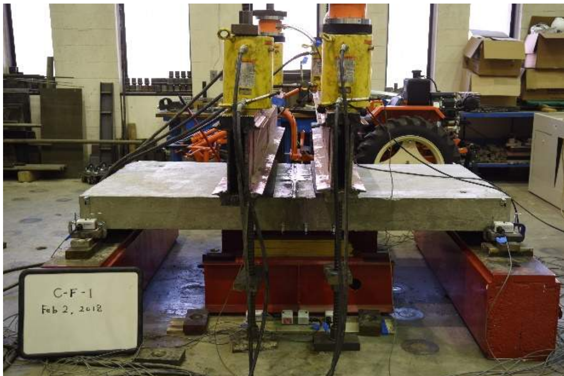
Figure 3.25: Four-point Bending Test Setup (Specimen C-F-1)
