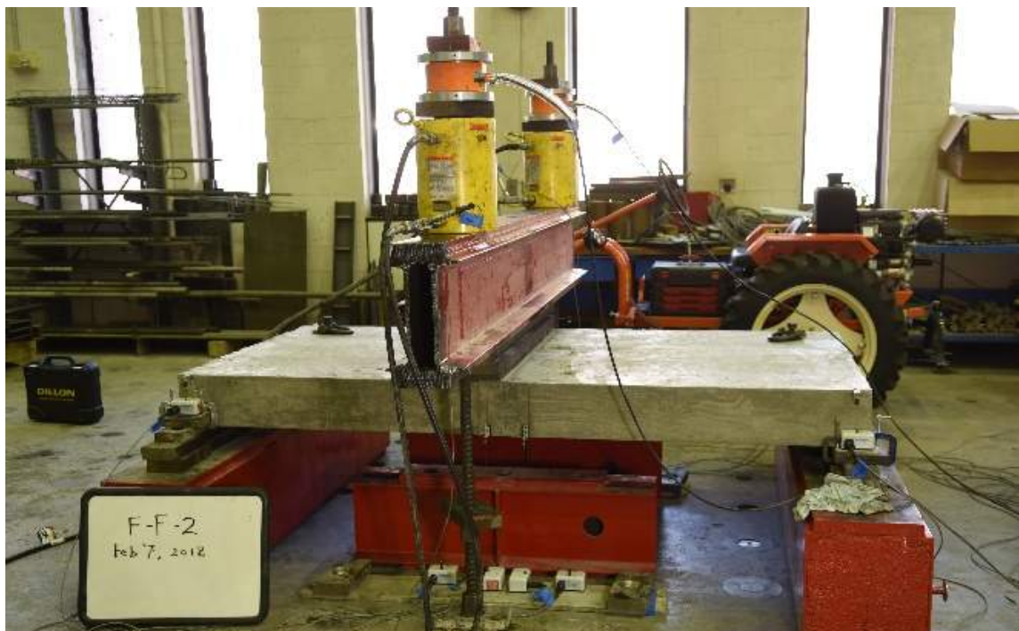
Figure 3.35: Three-point Bending Test Setup (Specimen F-F-2)
