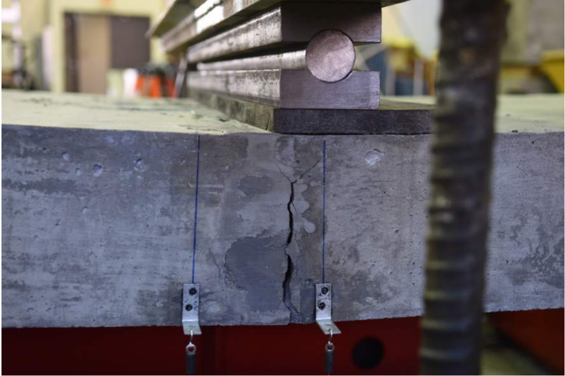
Figure 3.32: Crack Propagation (Specimen C-C-2)
