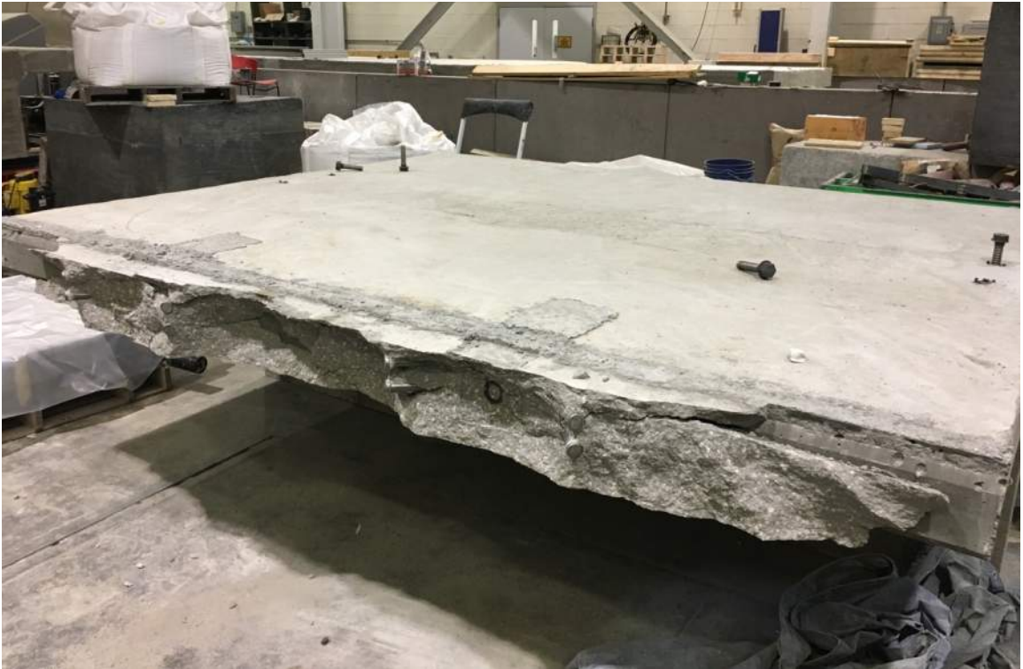
Figure 4.17: Grout Shear Key Bond Failure (Specimen F-M)
