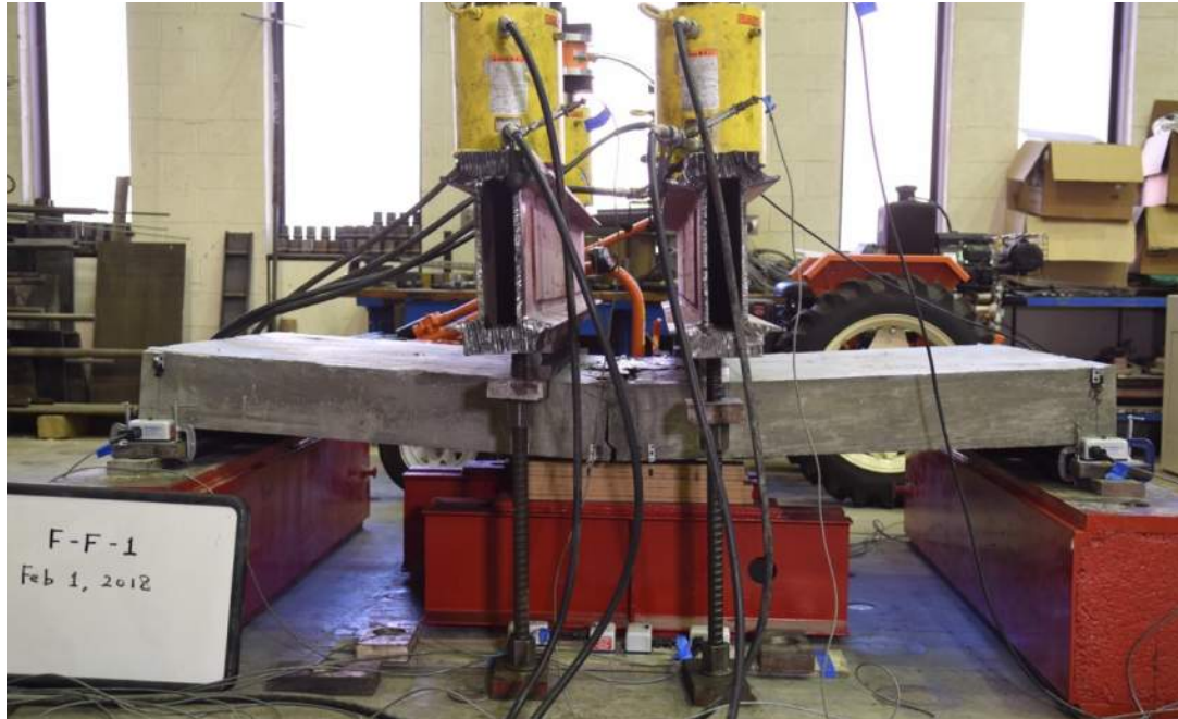
Figure 3.13: Concrete Crushing at Top (Specimen F-F-1)
