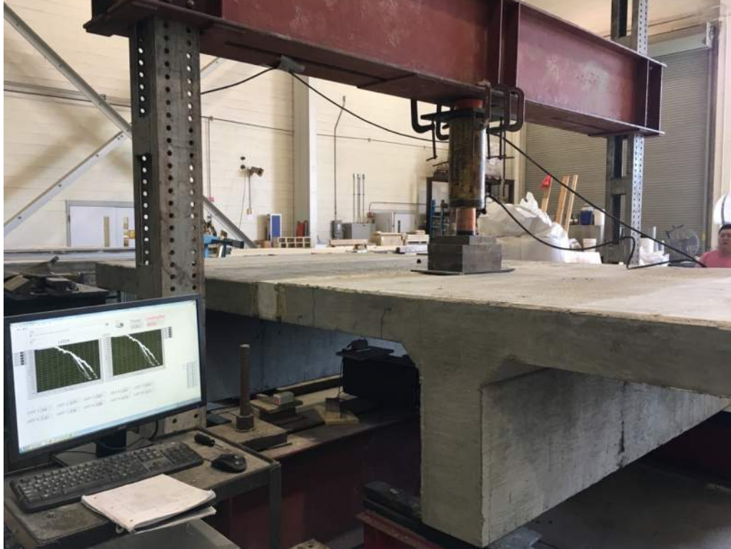
Figure 4.19: Test Setup and Loading of Specimen F-UHPC
