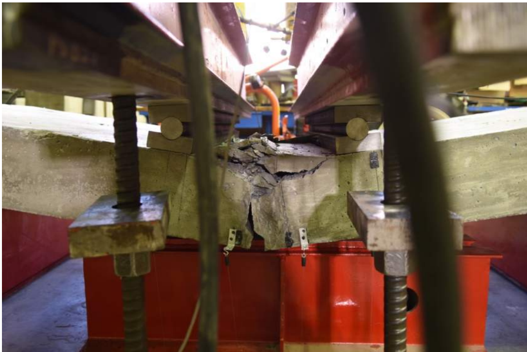
Figure 3.14: Grouted Joint Close-up Photo at Failure (Specimen F-F-1)
