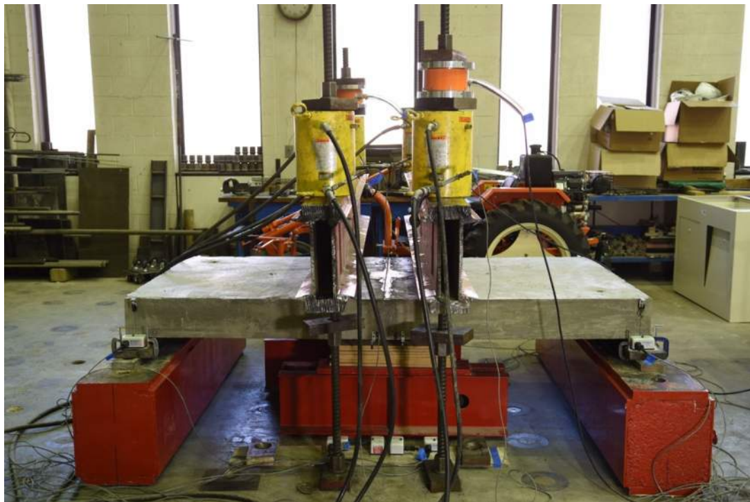
Figure 3.11: Four-point Bending Test Setup (Specimen F-F-1)
