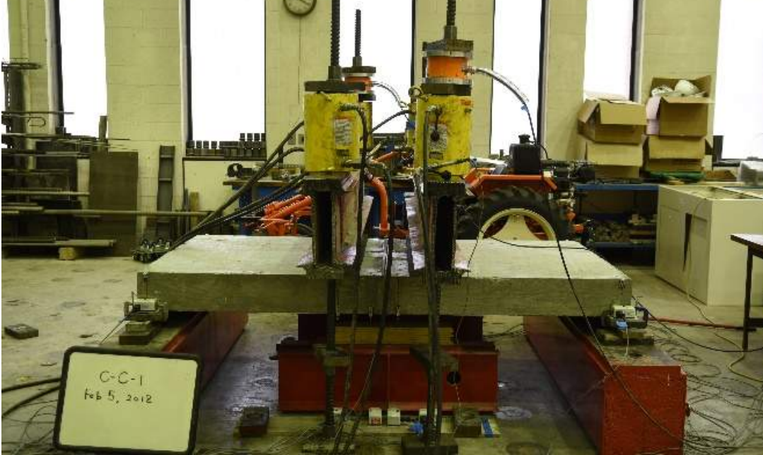
Figure 3.18: Four-point Bending Test Setup (Specimen C-C-1)
