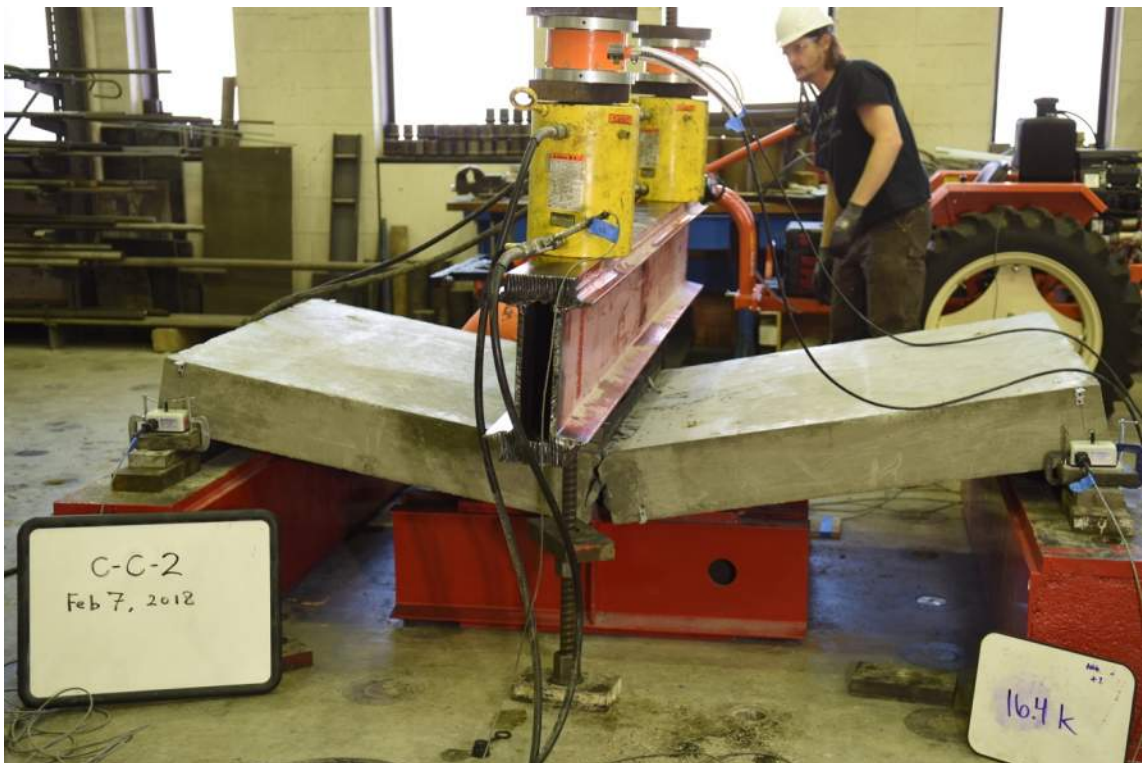
Figure 3.33: Specimen C-C-2 at Failure
