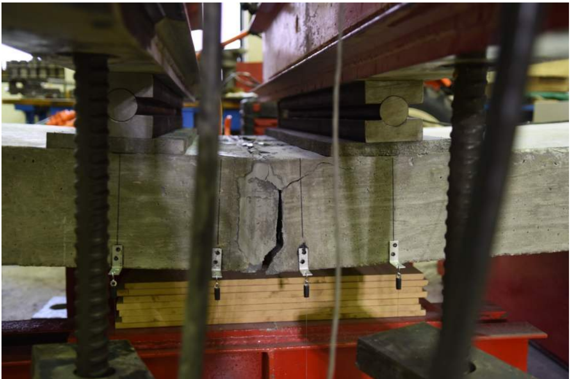
Figure 3.27: Crack Propagation (Specimen C-F-1)
