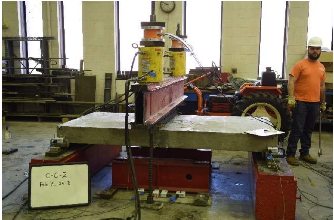
Figure 3.30: Three-point Bending Test Setup (Specimen C-C-2)
