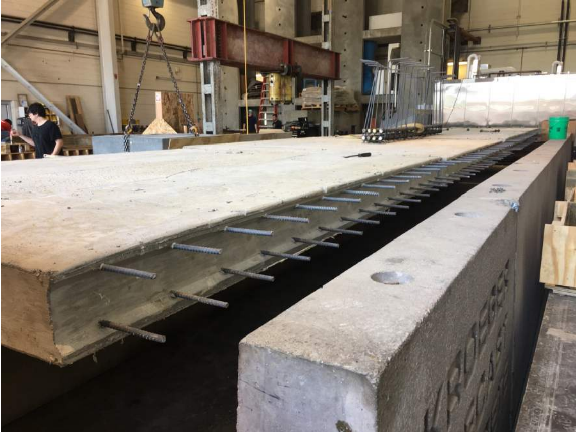
Figure 4.11: Test Specimens with Short Splice Length
