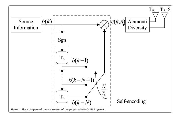
The spreading chips are then divided into two streams by applying Alam-outi scheme, where a block of two consecutive chips, c(k, 2i) and c(k, 2i + 1), are transmitted by sending c(k, 2i),  $-c^*(k, 2i + 1)$  to the first antenna, and c(k, 2i + 1),  $c^*(k, 2i)$  to the second antenna. Here,  $i \in \{0, 1, ..., N/2 - 1\}$  is the block index for the chips of the kth bit. The signals are then transmitted over a MIMO fading channel.
