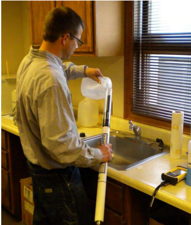
LLNRD staff calibrating a multi-parameter water quality meter
