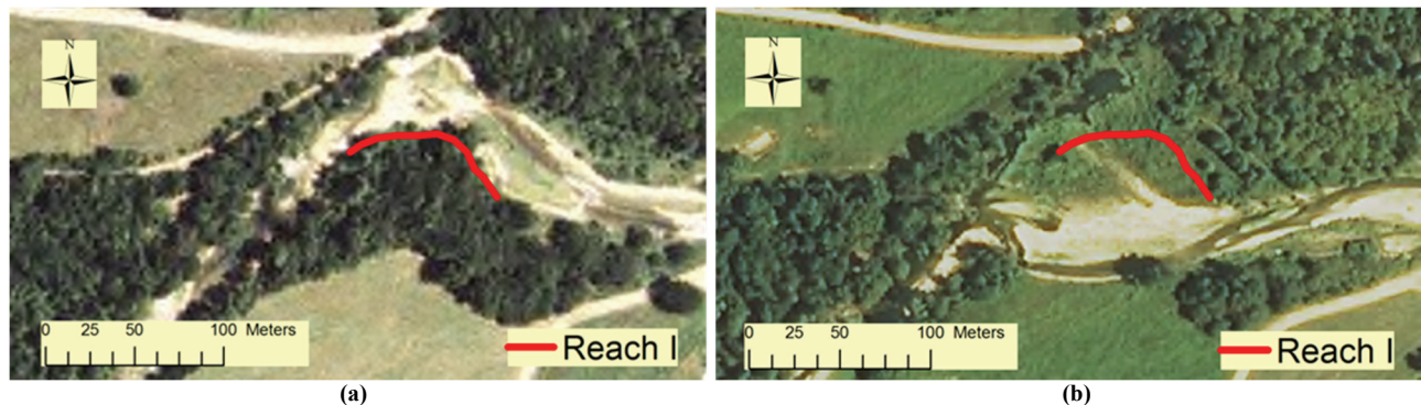
Figure 13. USDA National Agricultural Imagery Program aerial images showing streambank erosion from (a) 2003 to (b) 2013 for reach I on the Barren Fork Creek. The red line is the location of the reach in 2003.
