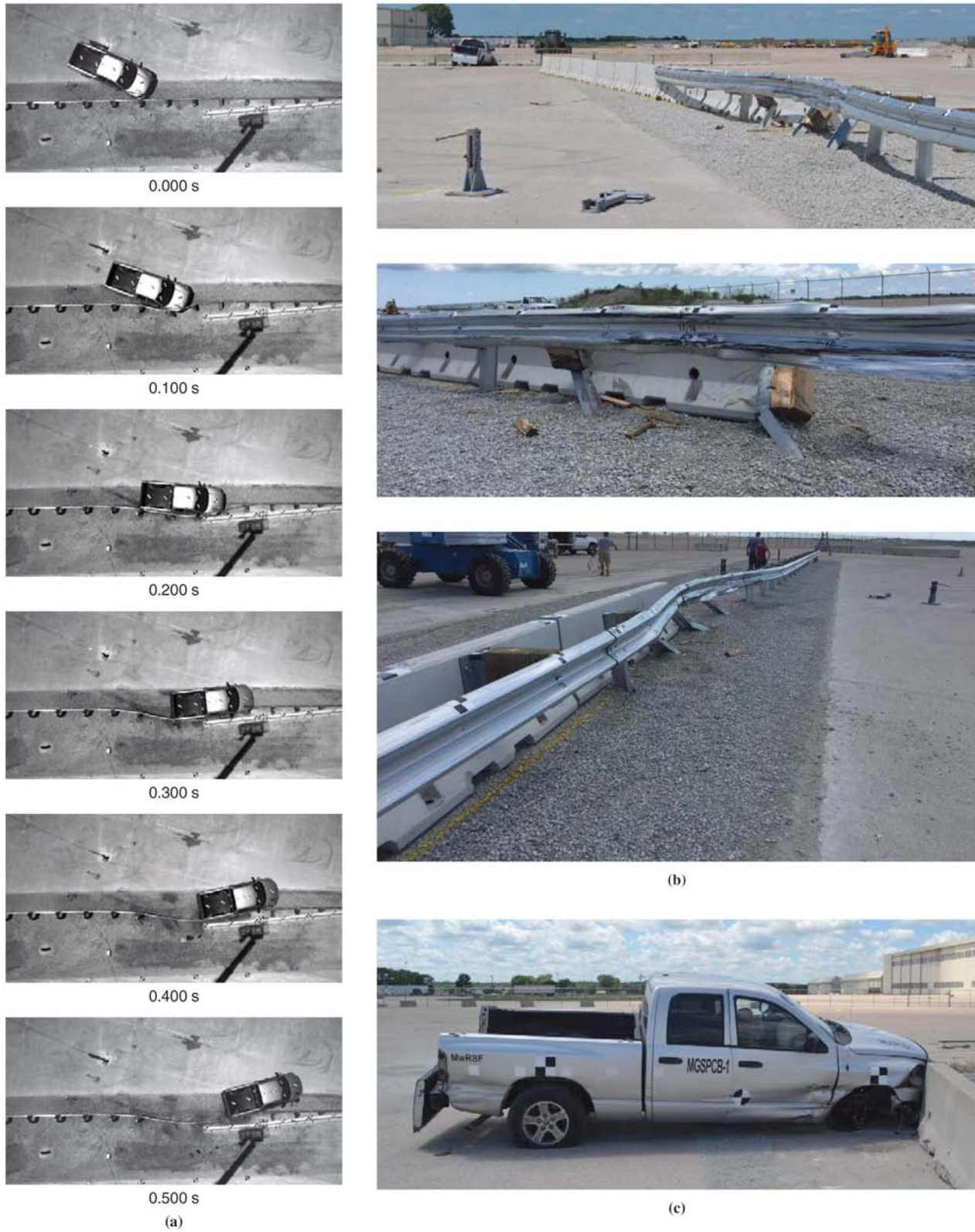
Figure 4. Test MGSPCB-1: (a) sequential events, (b) barrier damage, and (c) vehicle damage.
