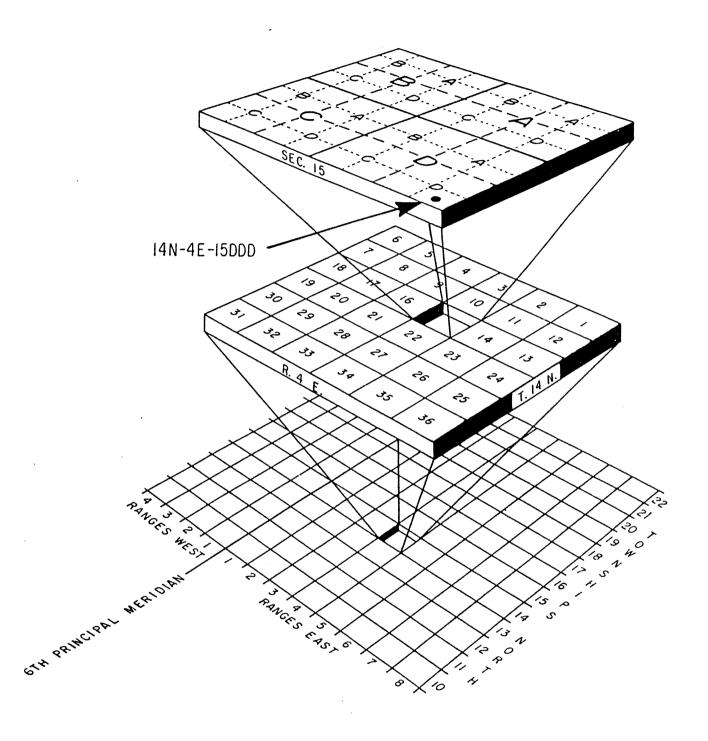
Fig. 1. System for identifying test-holes according to their location.
