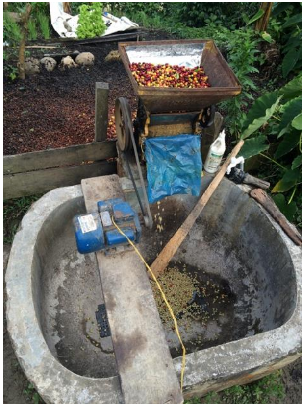
Figure 3. Motor-driven coffee pulper and tank
