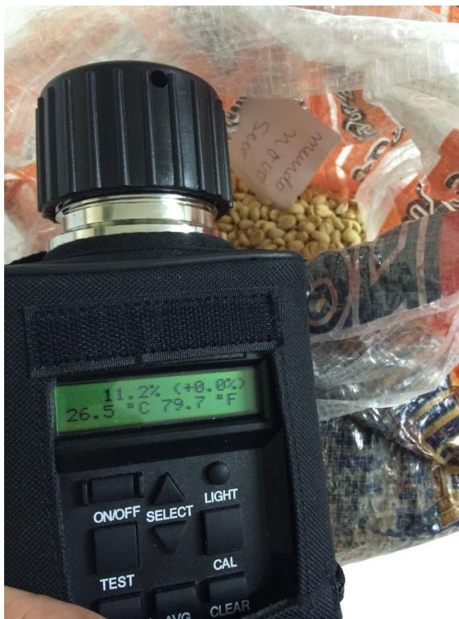
Figure 46. AgtraTronix 08150 handheld coffee moisture meter
