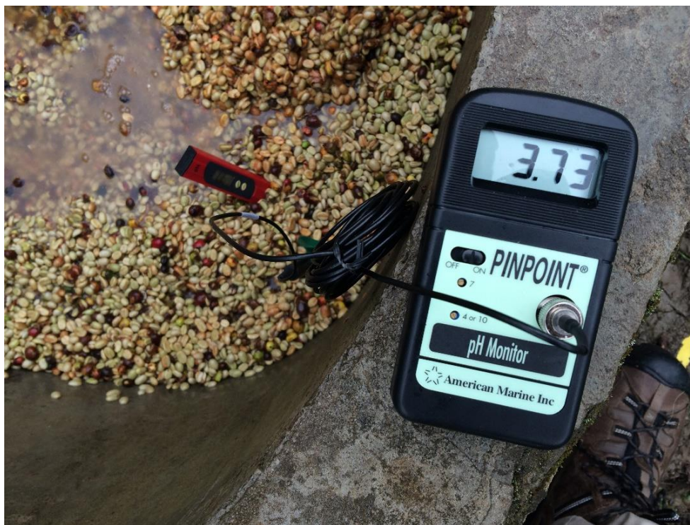
Figure 6. Monitoring fermentation with Pinpoint pH Monitor American Marine Inc.
