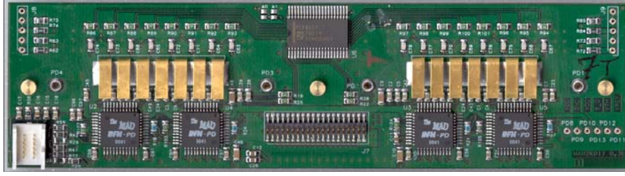
Figure 7.15: Front-end board (FEB).
