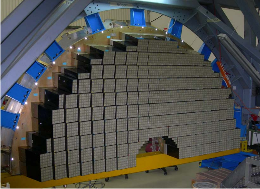
Figure 4.7: An endcap Dee, fully equipped with supercrystals.
