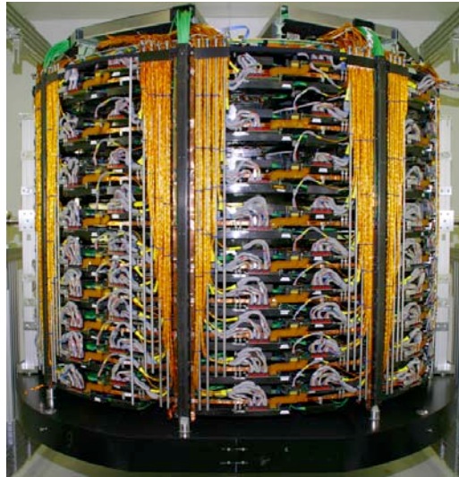
Figure 3.31: Side view of a TEC.
