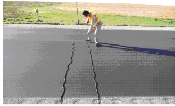
2. Fastening tube ends on the road
