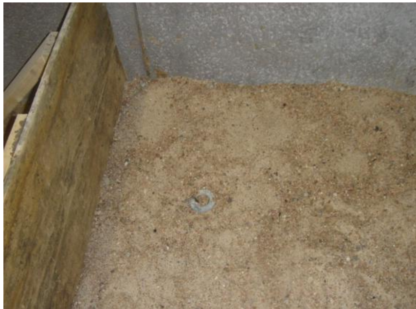
Figure 3.1 Metal ring placed underneath a 12 in. thick concrete slab
