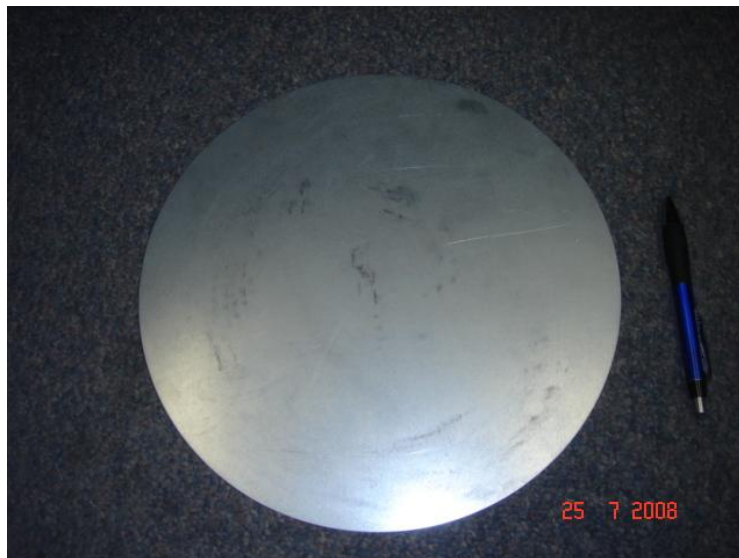
Figure 4.15 Steel plate placed underneath the concrete pavement
