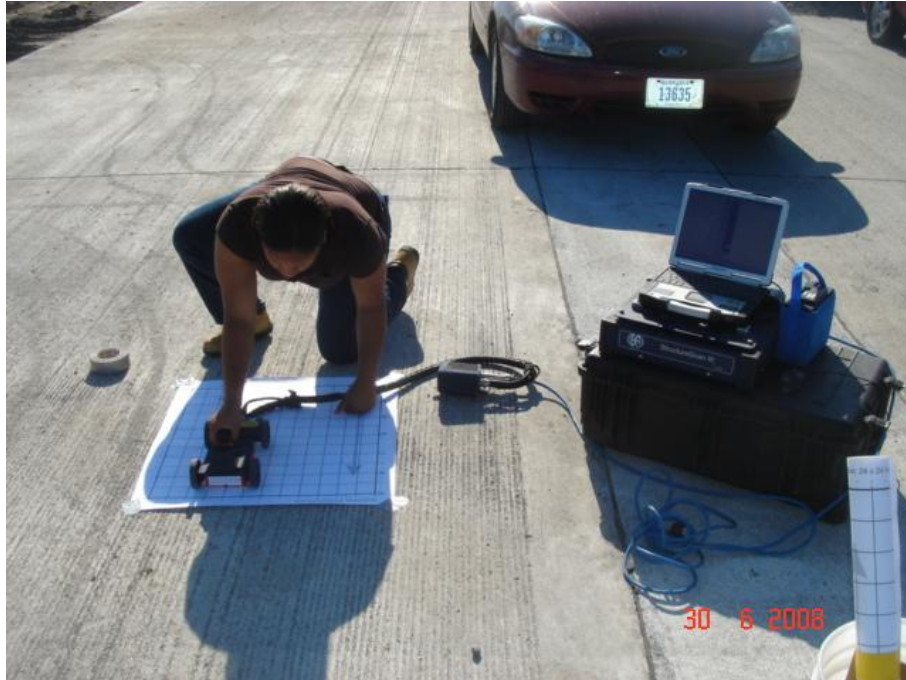
Figure 4.16 Grid scan at the marked location of the steel plate
