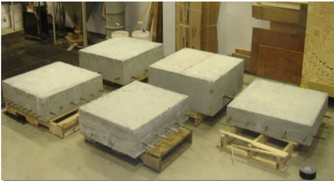
Figure 2.3: Reinforced Concrete Slabs Used for GPR Testing at PKI labs by authors
