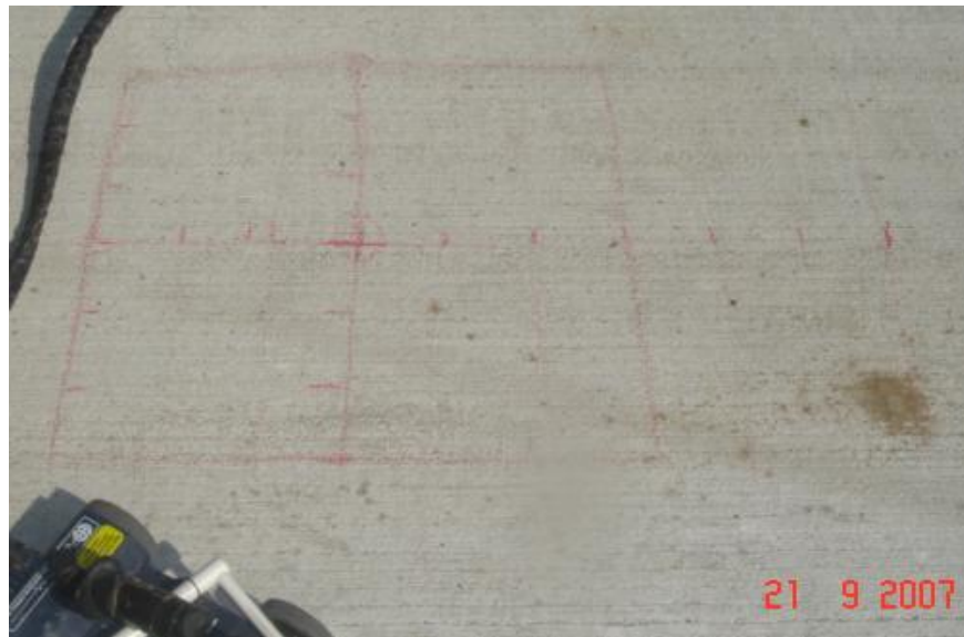
Figure 4.6 Grid used for scan # 1
