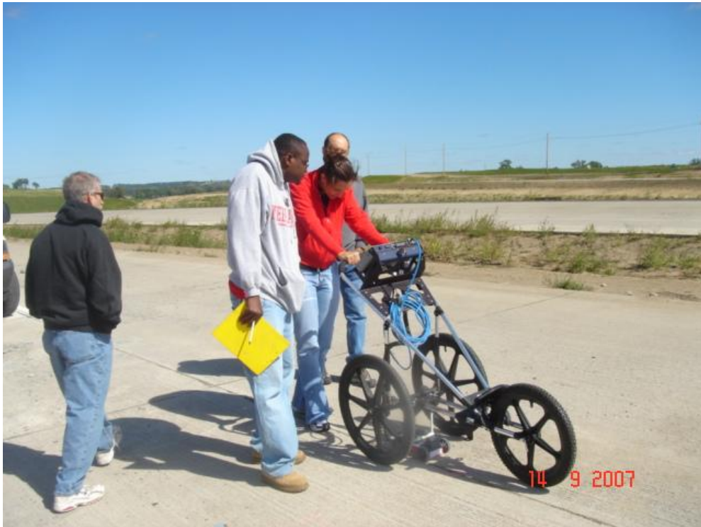
Figure 4.1 GPR scan using SIR 3000 system on highway I-275
