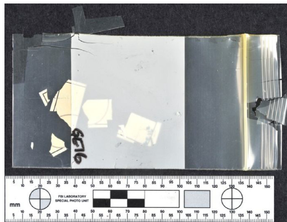
Fig. 6. Embrittlement of copier paper and degradation of polyethylene bag (90 kGy gamma).
