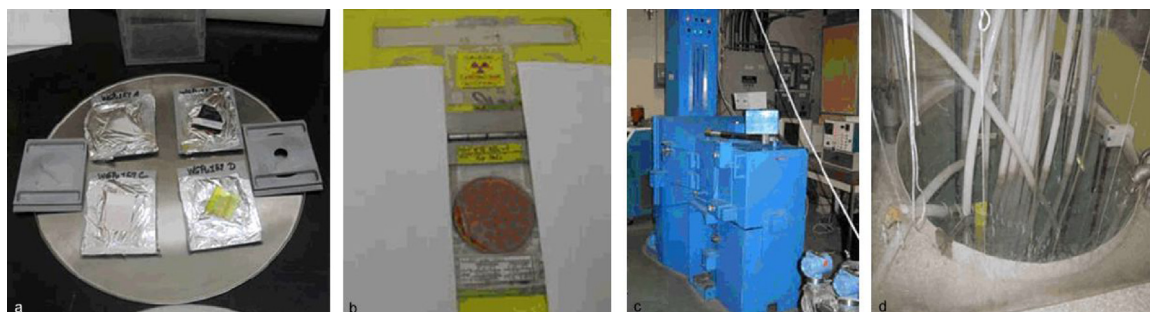
Fig. 1. Irradiation sources: (a) alpha planchet; (b) beta ^{90}\text{Sr}/^{90}\text{Y} ; (c) dry ^{60}\text{Co} irradiator; (d) SRNL neutron activation analysis facility.
