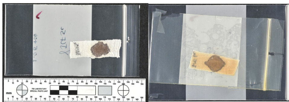
Fig. 7. Blood stains on cotton fabric after exposure to gamma irradiation at 9 kGy (left) and 90 kGy (right).
