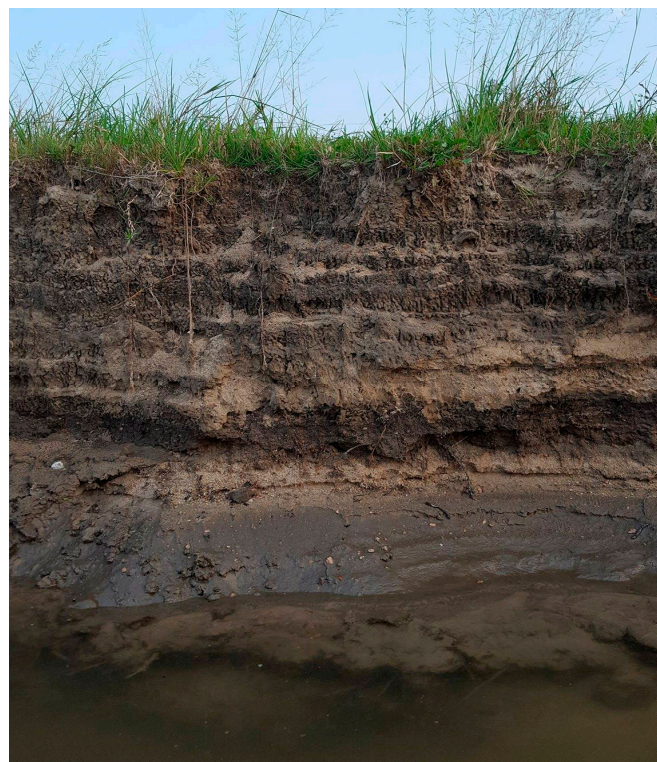
Figure 2. Typical streambank on Cedar River. Note the transition from sandy soil at the top to silty loam in the bottom.
