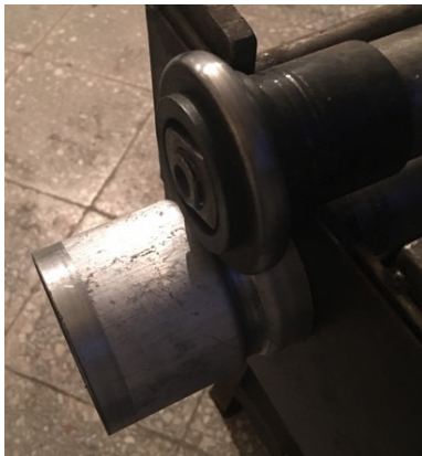
Figure 3: Stamping technique for fabrication of corrugations.
