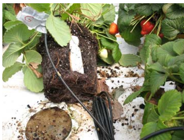
Figure 7b. Decagon GS3 sensor installed vertically across the root mass inside of the pot.
