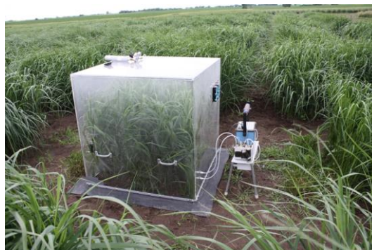
Fig 1. Performance evaluation of the constructed plexiglass chamber without and with enclosed plants. A (Top). Labeling chamber dimensions were 1.0×1.0×0.0016 m. The main components of the system were (A) CO 2 sampling ports, (B) air circulation fans, (C) CO 2 injection port, (D) Li-6200. Figure 1B (Bottom). Labeling chamber in a typical field setting over a switchgrass plot.
