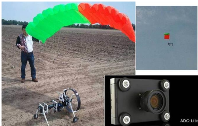
Figure 4 Hawkeye UAV with ADC-Lite multispectral camera (Tetracam, Inc., Chatsworth, CA, USA)
