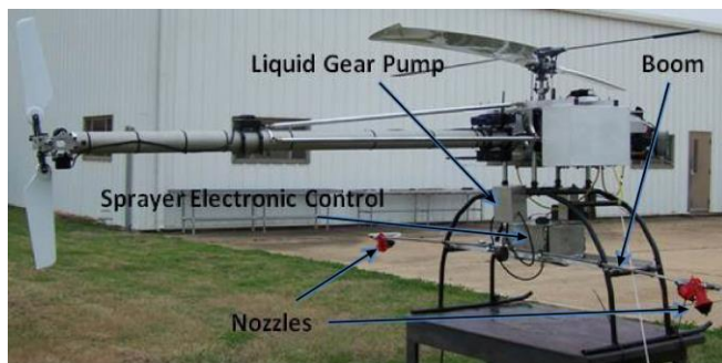
Figure 1 A low-volume spray system integrated with a UAV
