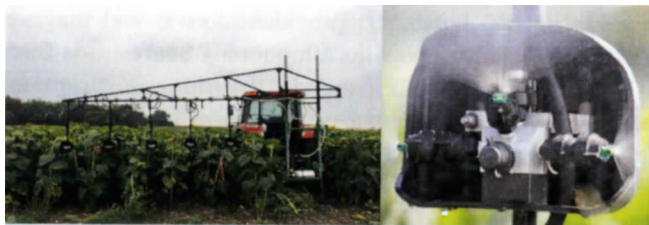
Figure 13.2 Small-plot ground rig equipped with 360 Undercover® drop nozzles (360 Yield Center, LLC; Morton, IL) to apply avian repellent under the crop canopy and increase application to targeted area (e.g., sunflower face or corn husk). Use of trade names does not imply endorsement by the U.S. government. (Courtesy of Page Klug/USDA Wildlife Services; and 360 Yield Center, https://360yieldcenter.com/products/360-undercover/ .)
