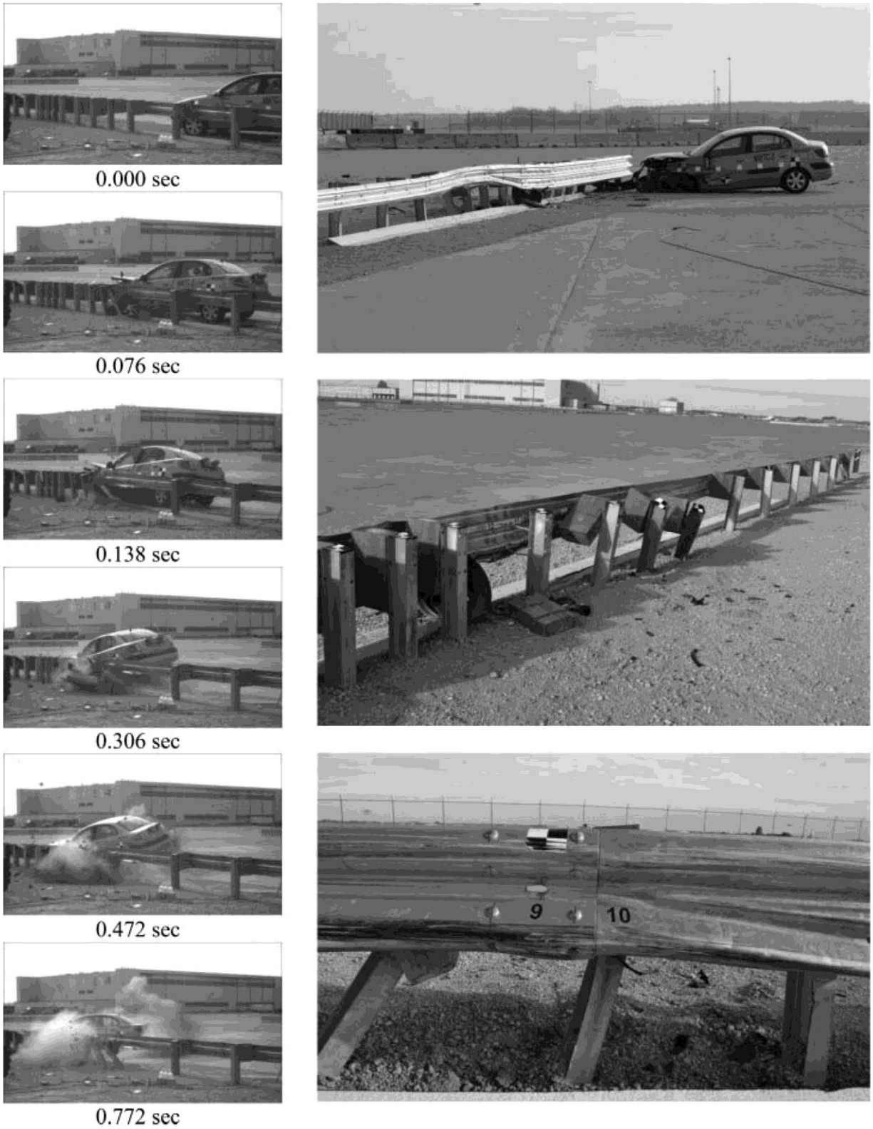
Fig. 7. Sequential photos and system damage, Test No. MWTC-2 (Winkelbauer et al., 2014).
