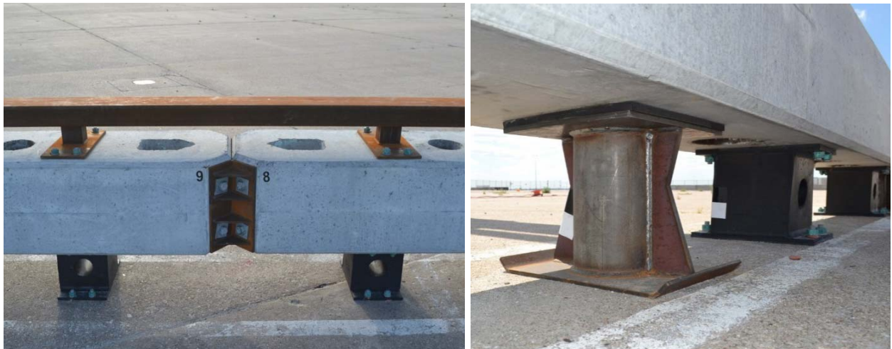
FIGURE 1 View of initial concept with elastomer posts and metal skins (4,14).
