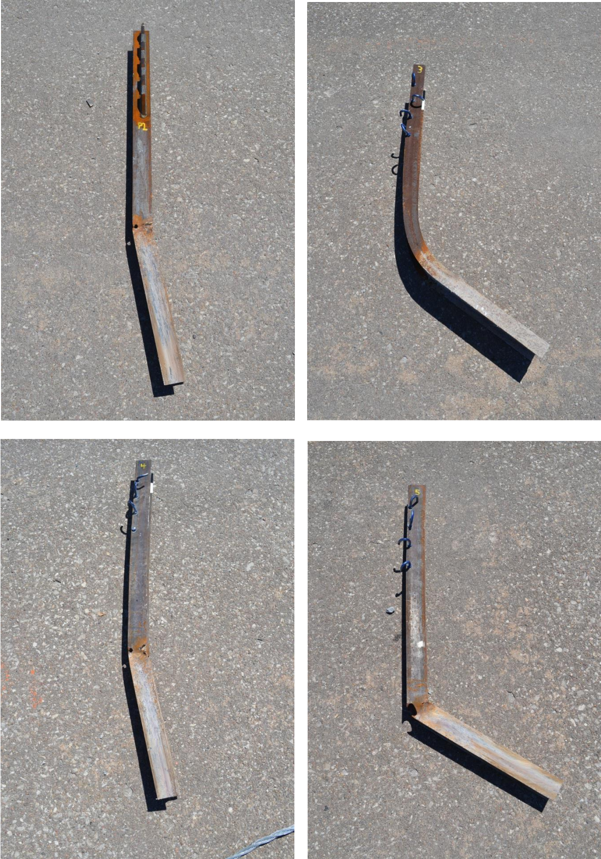
Figure 28. System Damage – Post Nos. 2 through 5, Test No. HTCT-2
