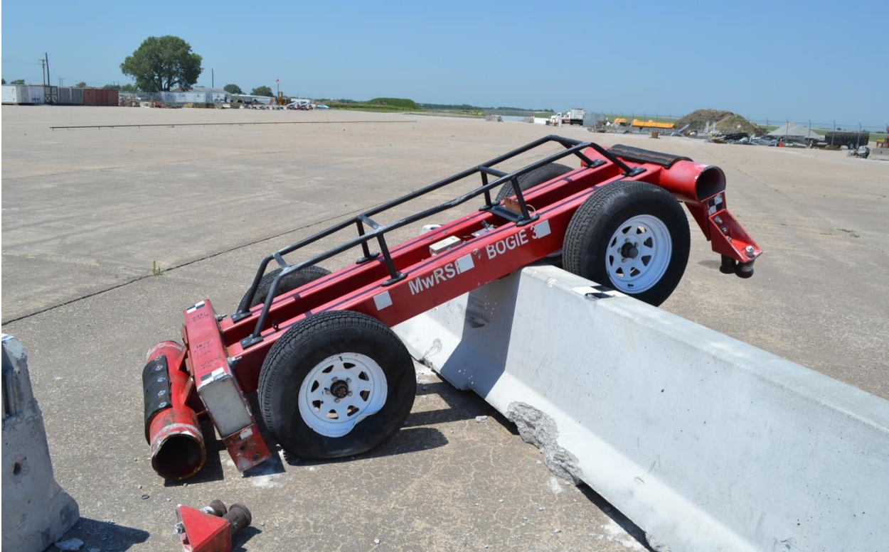
Figure 40. Bogie Damage, Test No. HTCT-3
