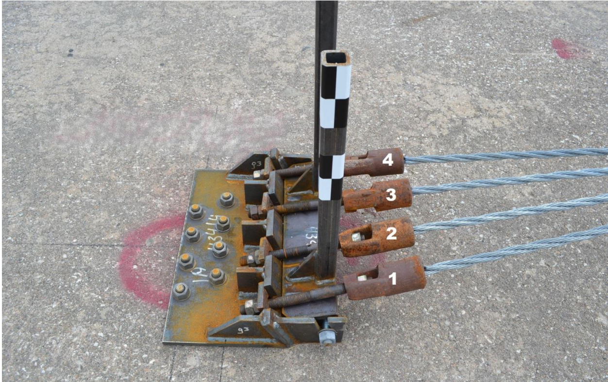
Figure 23. Cable Numbers at Upstream Cable Anchor Bracket, Test No. HTCT-2
