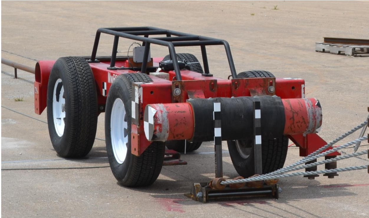
Figure 21. Rigid Frame Bogie on Guidance Track
