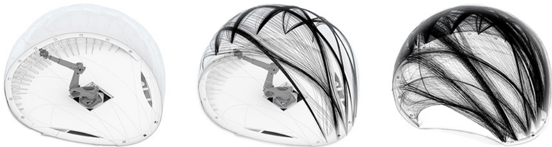
Figure 2.10 Robotic fabrication from the inside of the ETFE shell, robot arms lays carbon fibers by using a computational agent-based design (Menges et al 2014). Retrieved from: https://www.designboom.com/architecture/icd-itke-research-pavilion-2014-15-water-spider-07-16-2015/
