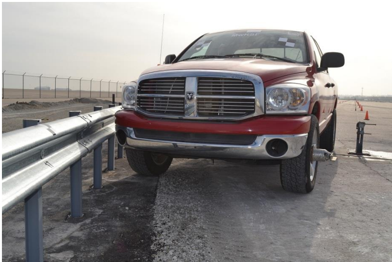
Figure 80. Impact Location, Test No. MGSMS-1
