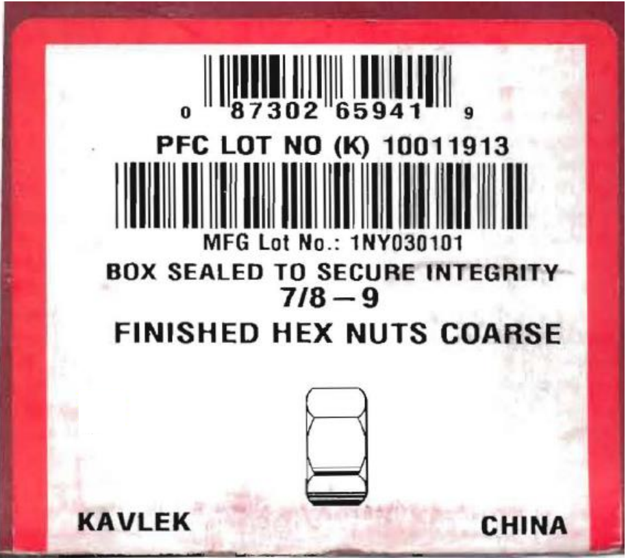
Figure C-21. 7/8-in. Dia. x 8-in Hex Bolt and Nut Material Specs, Test No. MGSMS-1
