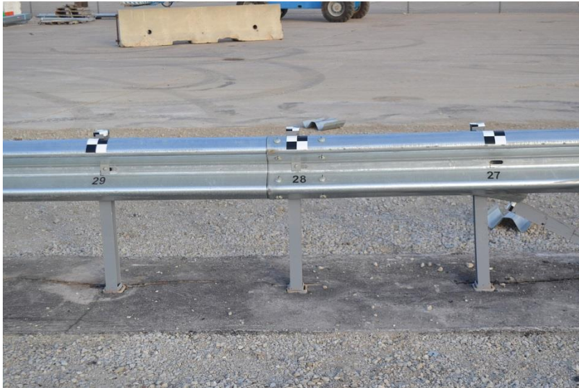
Figure 86. System Damage – Post Nos. 24 Through 29, Test No. MGSMS-1
