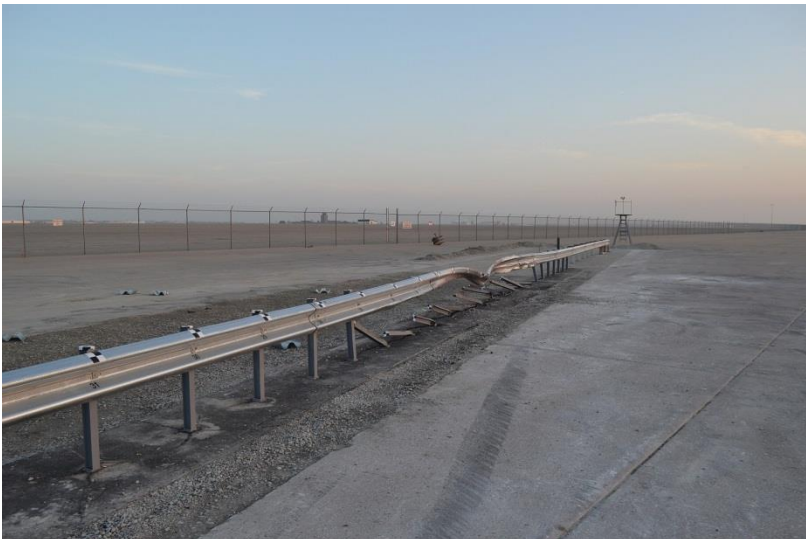
Figure 82. System Damage, Test No. MGSMS-1
