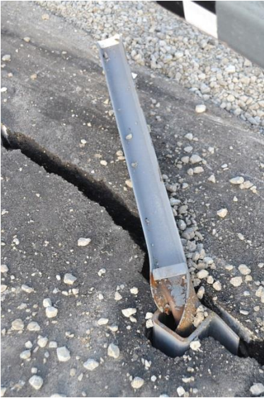
Figure 85. System Damage – Post Nos. 21 Through 23, Test No. MGSMS-1
