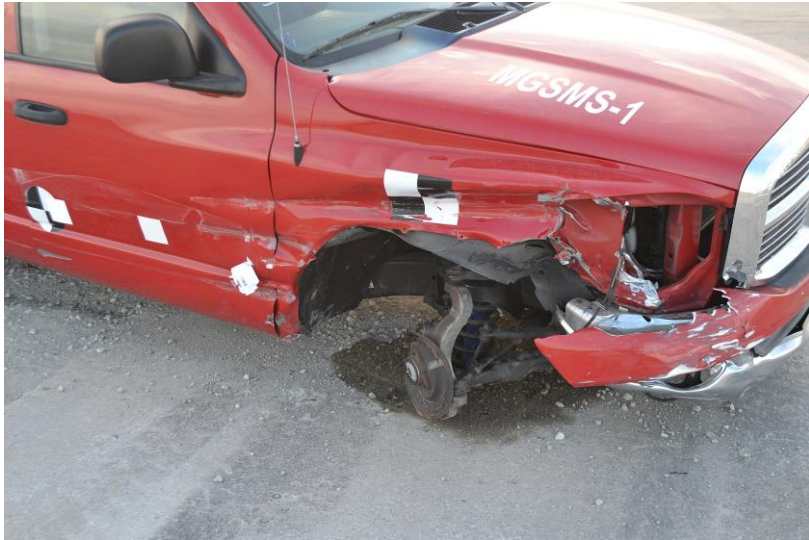
Figure 89. Vehicle Damage, Test No. MGSMS-1
