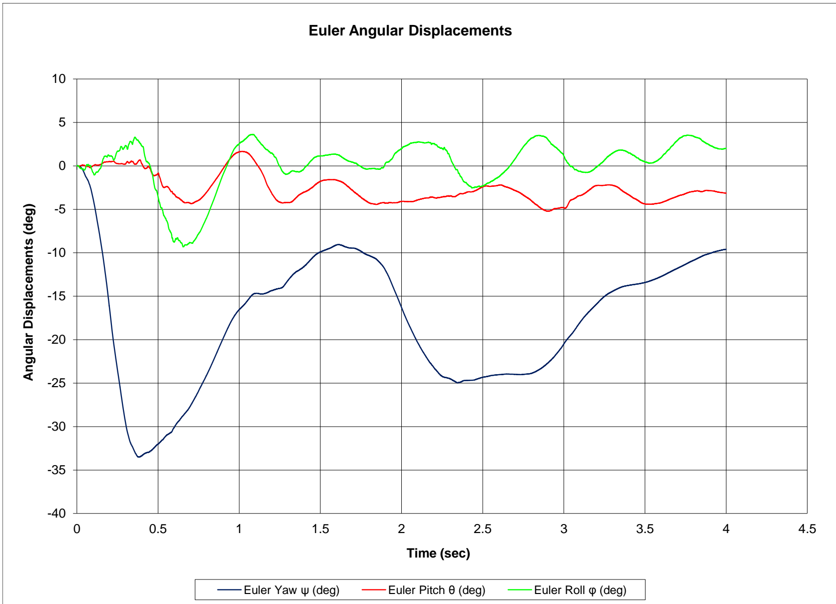
Figure G-7. Vehicle Angular Displacements (SLICE-2), Test No. MGSMS-1
