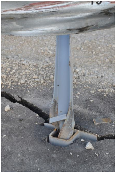
Figure 84. System Damage – Post Nos. 18 Through 20, Test No. MGSMS-1
