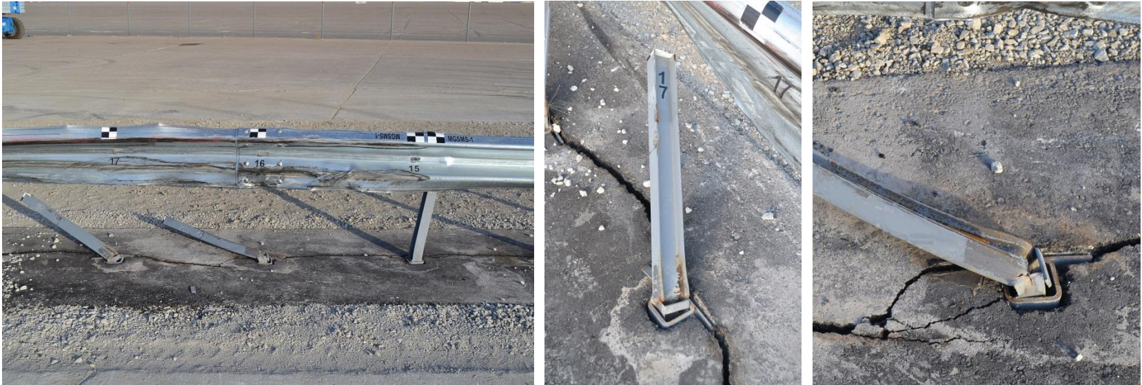
Figure 83. System Damage – Post Nos. 12 Through 17, Test No. MGSMS-1
