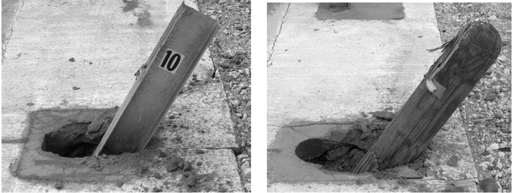
Figure 1. Pre- and Post-Test Photos of Posts in Grout-Filled Leave-Outs [3]
