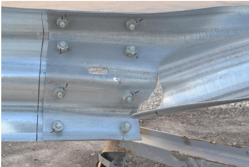
Figure 88. System Damage – Rail Tearing, Test No. MGSMS-1
