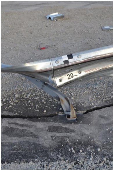
Figure 84. System Damage – Post Nos. 18 Through 20, Test No. MGSMS-1
