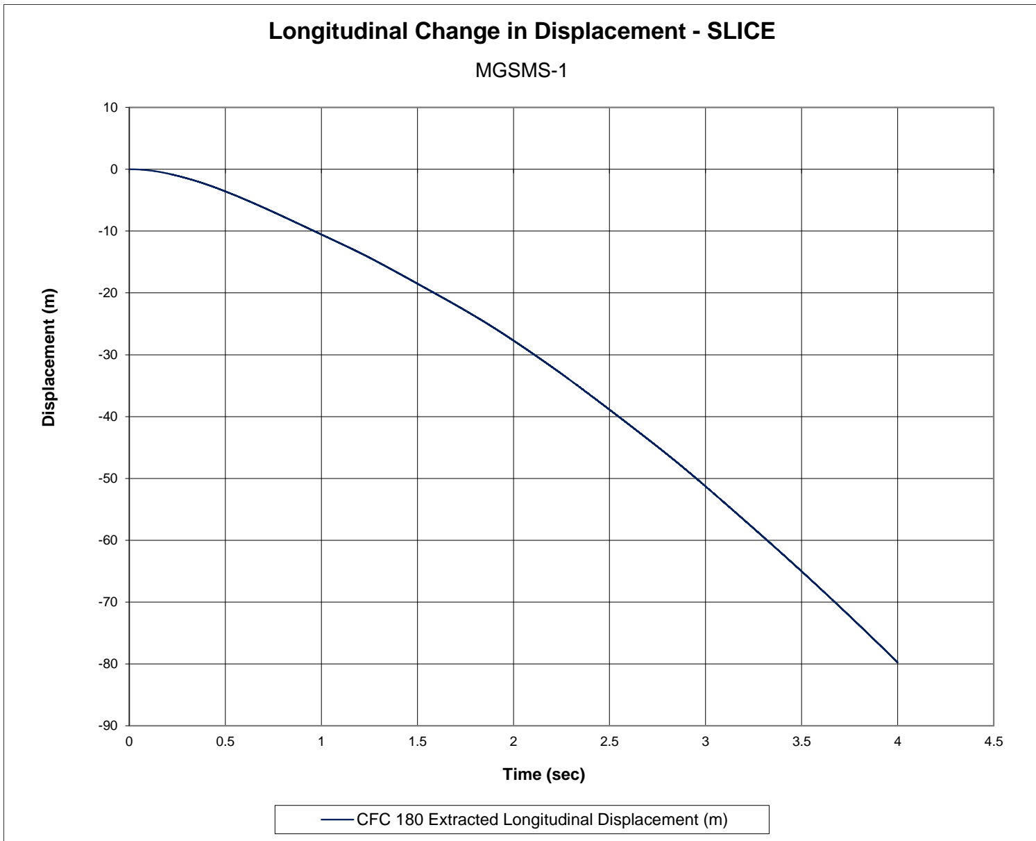
Figure G-3. Longitudinal Change in Displacement (SLICE-2), Test No. MGSMS-1
