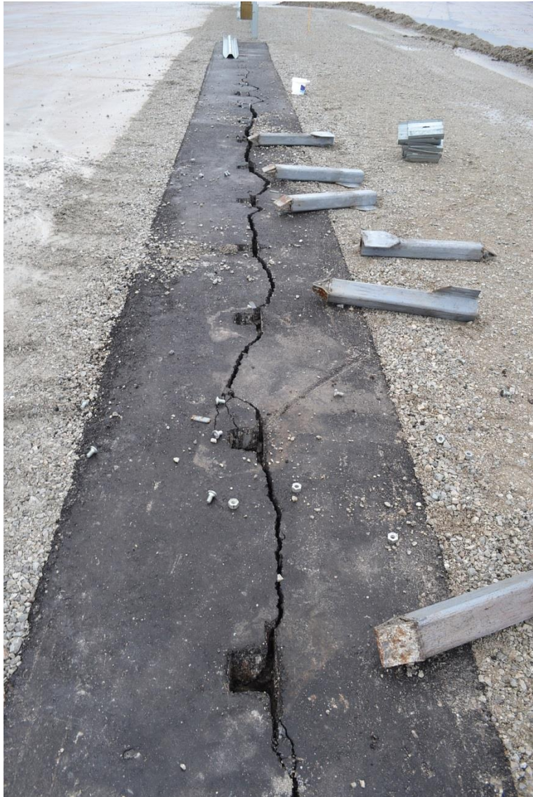
Figure 87. System Damage – Asphalt Fracture and Anchor Movement, Test No. MGSMS-1
