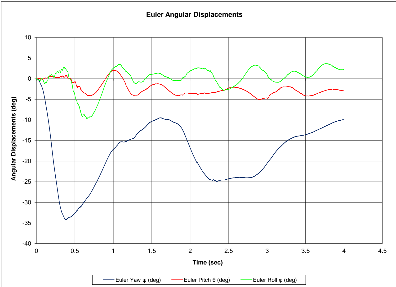
Figure G-15. Vehicle Angular Displacements (DTS), Test No. MGSMS-1
