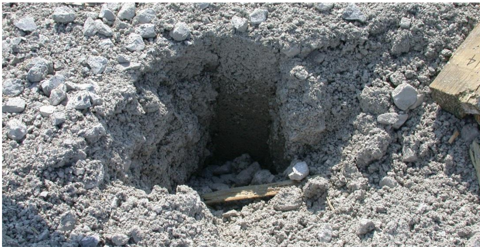
Figure 17. Post No. 16 Pulled Out of Ground, Test No. NPG-5
