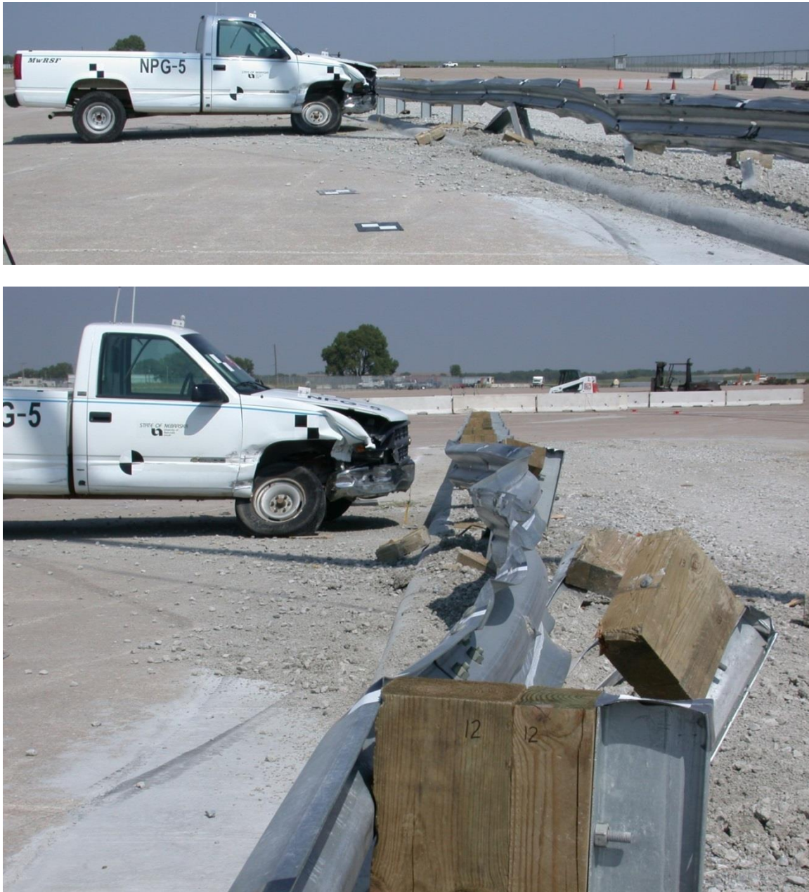
Figure 16. System Damage, Test No. NPG-5
