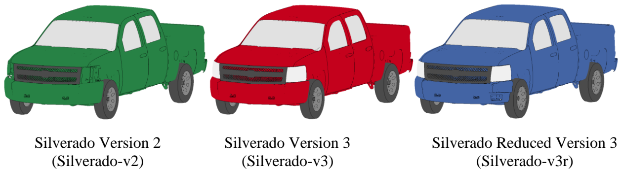
Figure 1. Computer Simulation Models of 2270P Chevrolet Silverado Pickup Trucks
