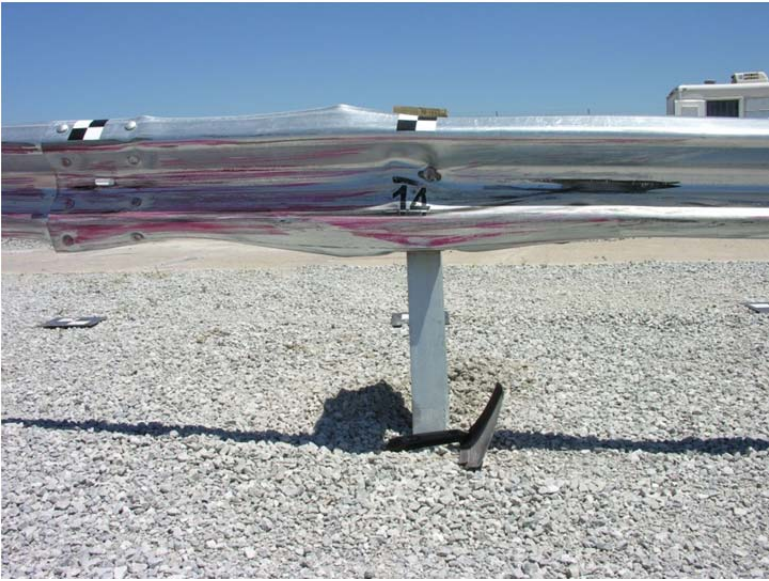
Figure 43. Post Nos. 13 and 14 Damage, Test No. MGSMRH-1
