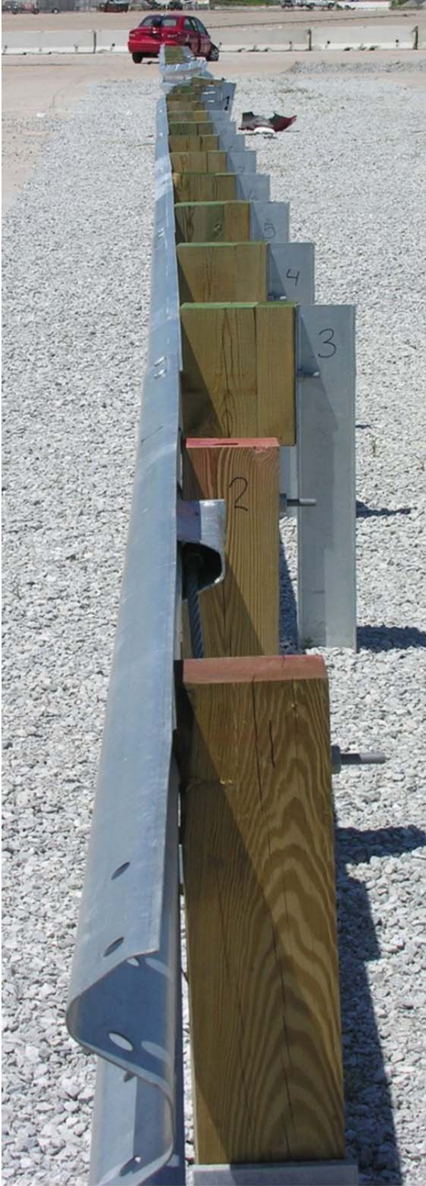
Figure 37. System Damage, Test No. MGSMRH-1
