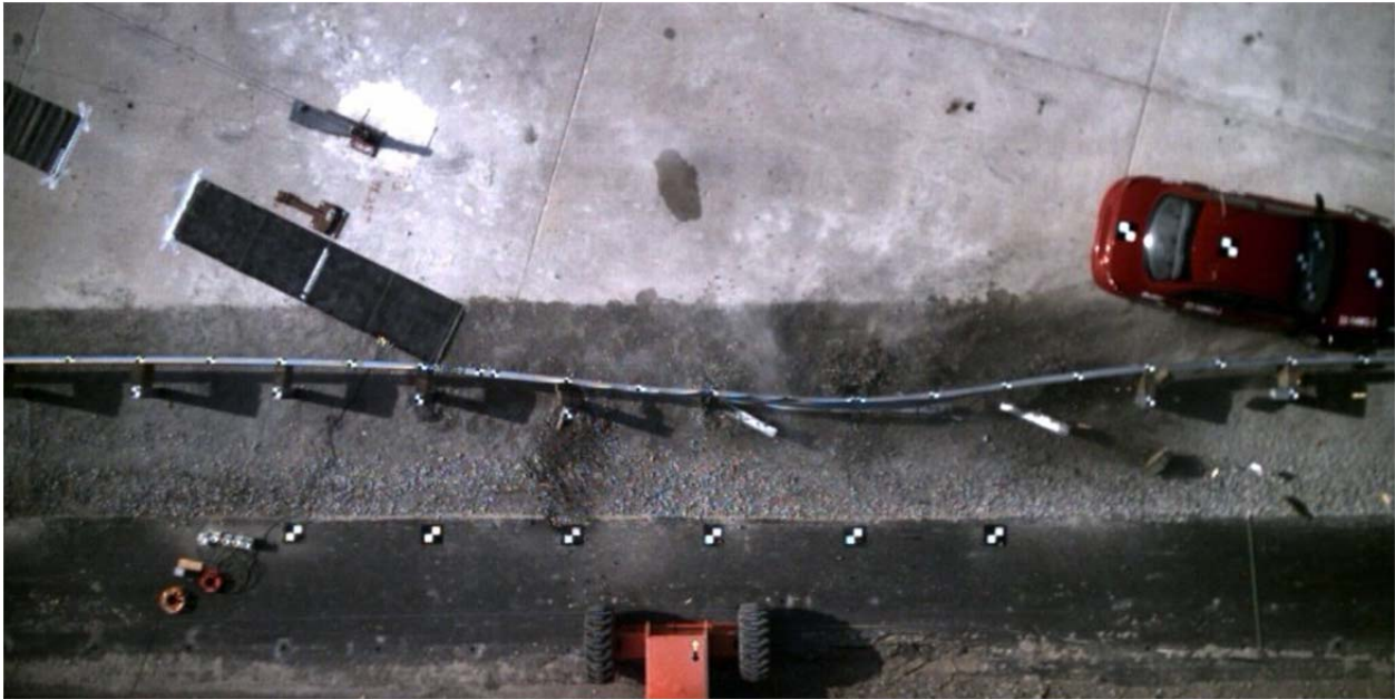
Figure 4. Test No. 2214MG-3, Vehicle Yaws Toward the Barrier
