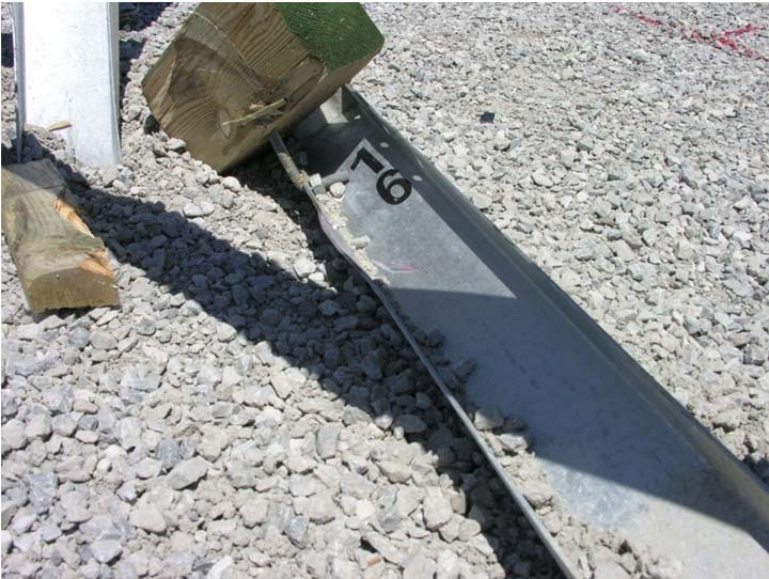
Figure 44. Post Nos. 15 and 16 Damage, Test No. MGSMRH-1
