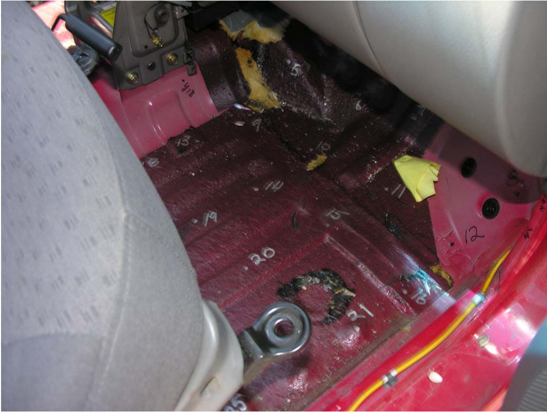
Figure 48. Occupant Compartment Damage, Test No. MGSMRH-1
