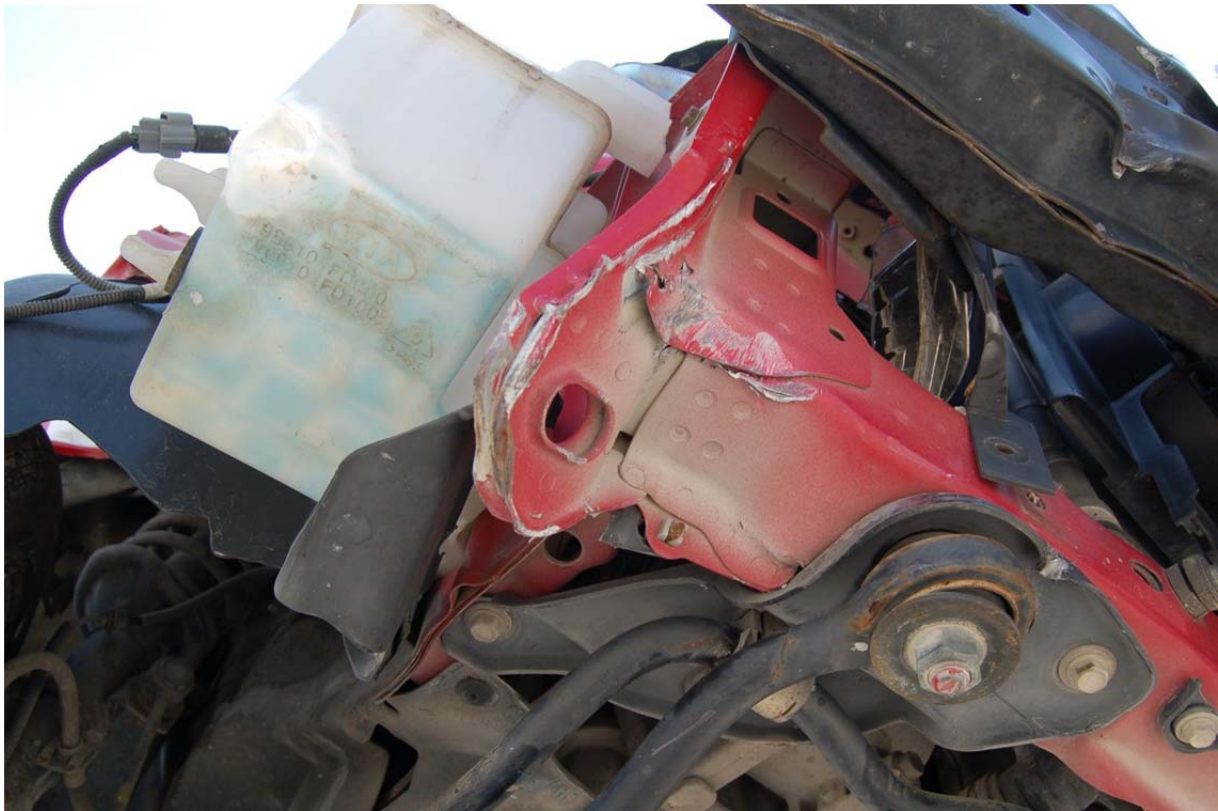
Figure 49. Undercarriage Damage, Test No. MGSMRH-1
