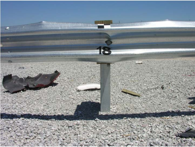
Figure 45. Post Nos. 17 and 18 Damage, Test No. MGSMRH-1
