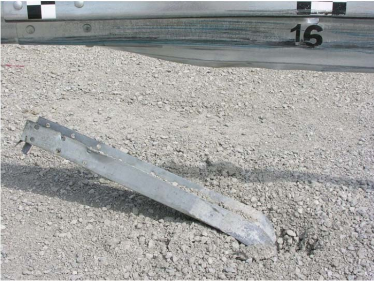
Figure 66. Post Damage, Test No. MGSMRH-2
