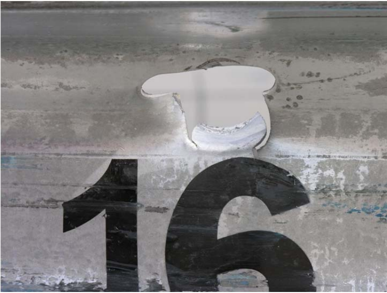
Figure 64. Post-To-Rail Bolt Hole Damage, Test No. MGSMRH-2
