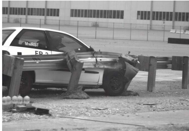
Figure 1. Test No. FR-3, Potential for Wheel Snag
