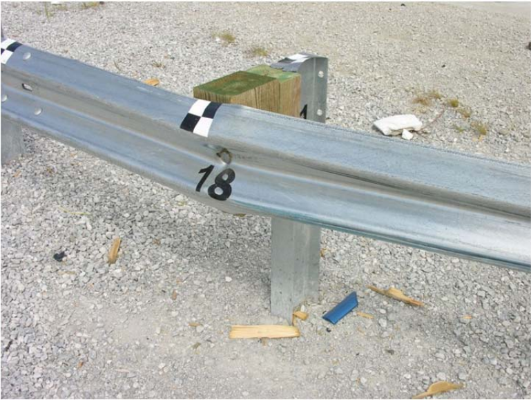
Figure 67. Post Damage, Test No. MGSMRH-2
