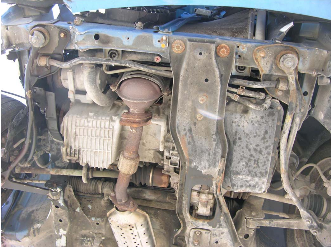
Figure 71. Undercarriage Damage, Test No. MGSMRH-2
