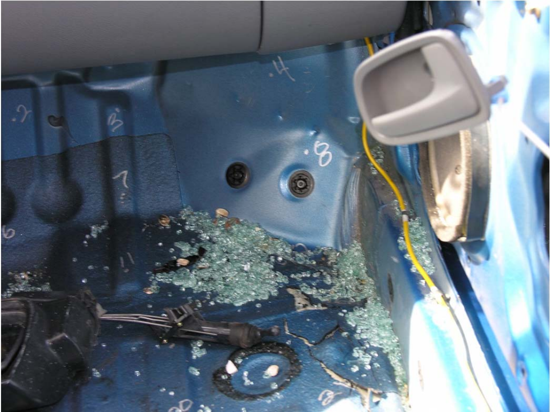
Figure 70. Occupant Compartment Damage, Test No. MGSMRH-2
