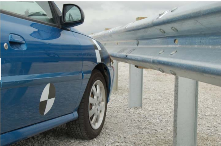
Figure 8. 1100C Next to 32-, 34-, and 36-in. (813-, 864-, and 914-mm) MGS – Rear View
