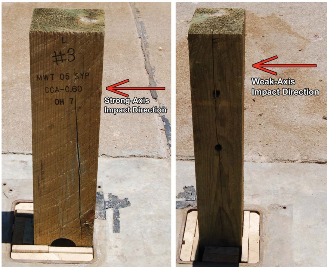
Fig. 4. Model CRT and post impact configurations.
