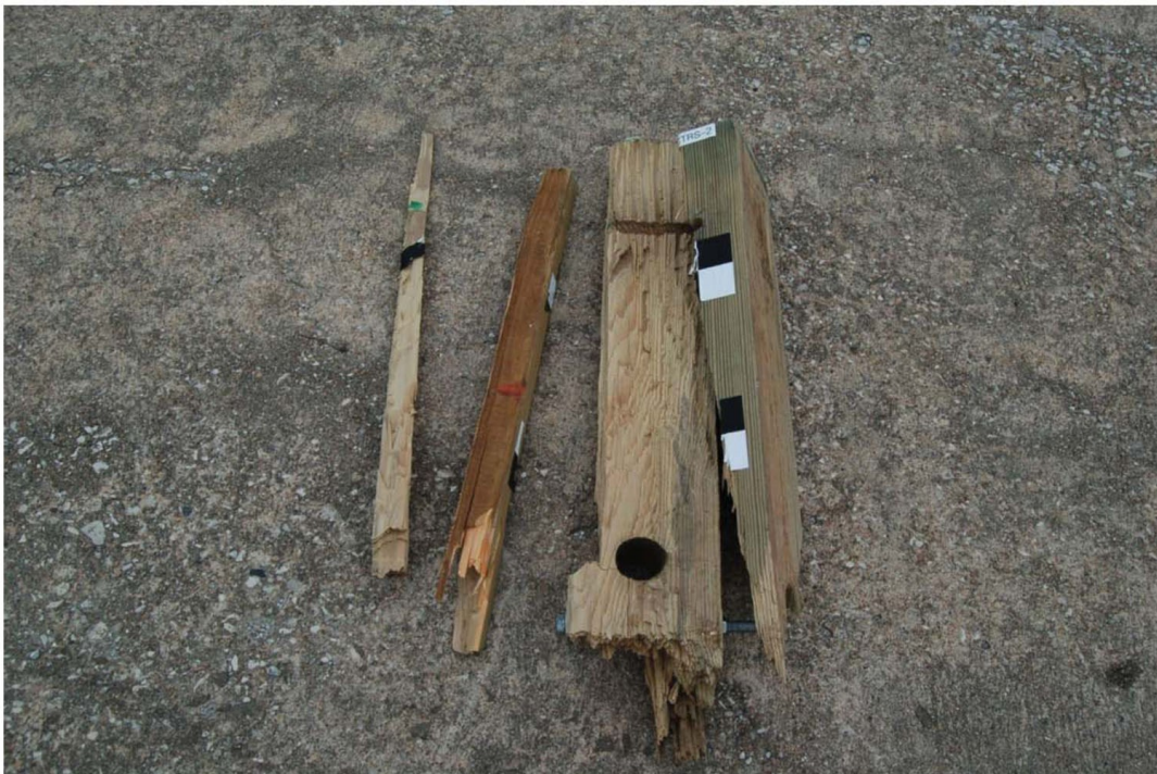
Fig. 8. Post splitting bogie component testing, before and after impact.
