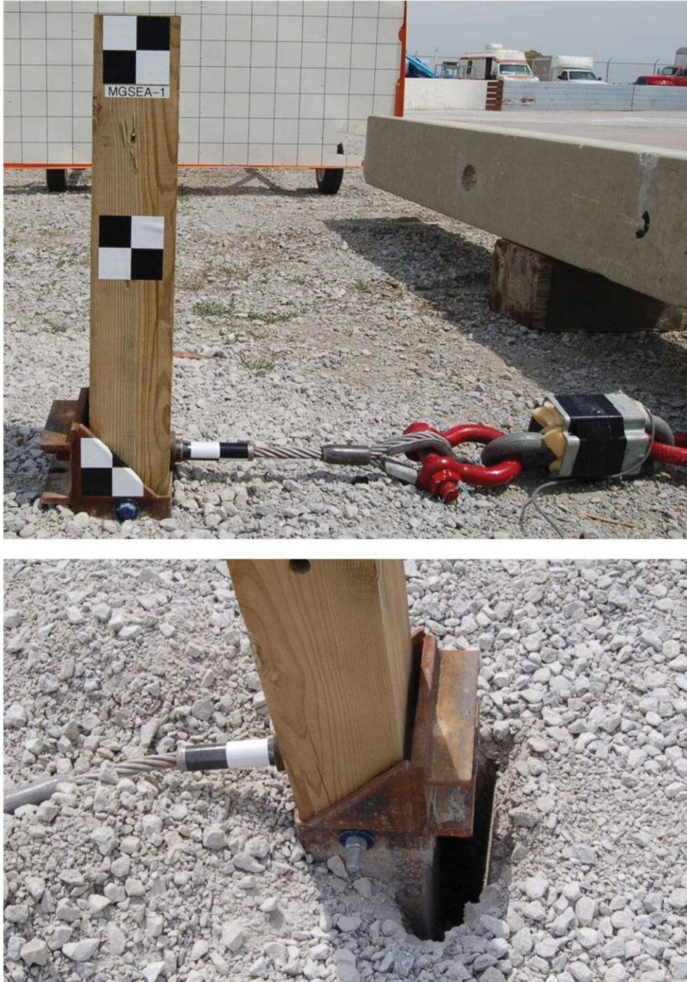
Fig. 2. Soil foundation tube pull test setup, before and after test.
