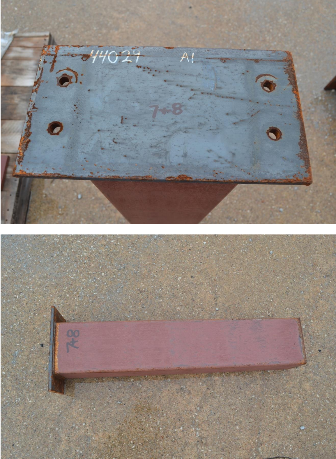
Figure 37. Lower Section and Base Plate, Test No. UBSPB-8
