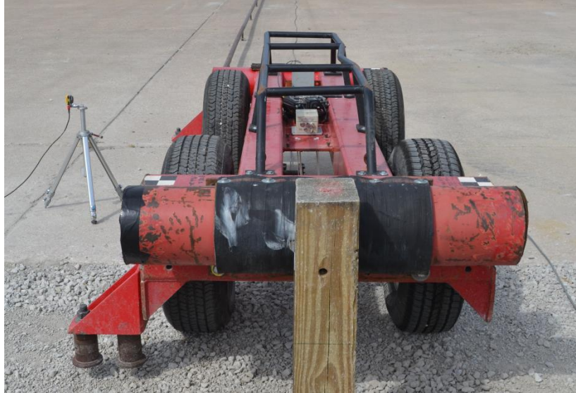
Figure 2. Rigid Frame Bogie and Guidance Track
