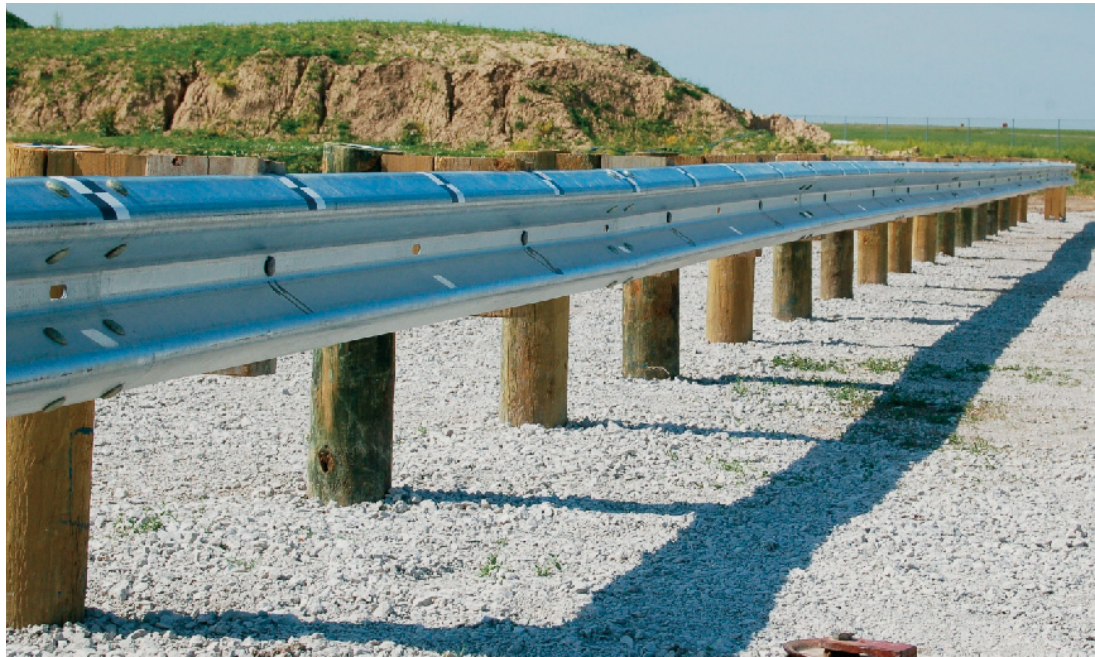
FIGURE 4 Test installation of MGS with round wood posts (BCT = breakaway cable terminal).
