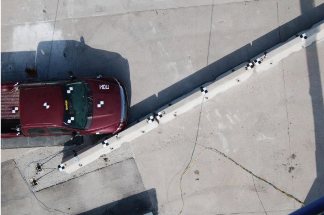
Figure 31. Impact Location, Test No. TTCB-1
