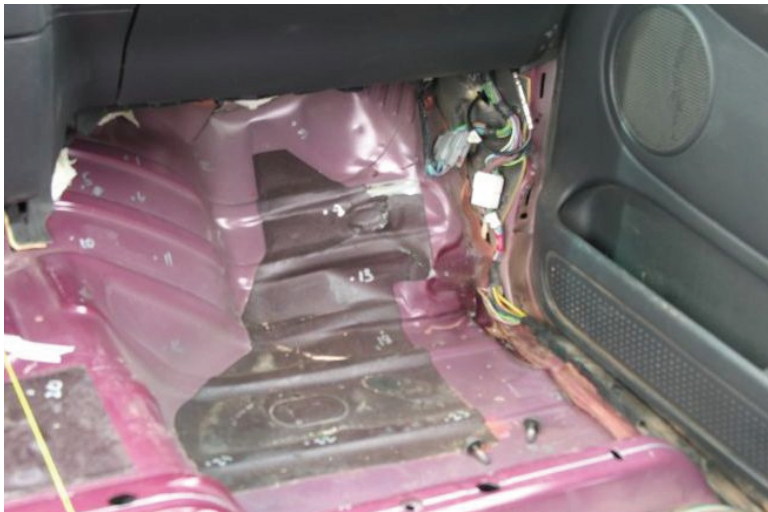
Figure 45. Vehicle Damage, Occupant Compartment, Test No. TTCB-1
