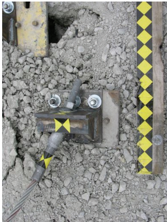
Figure 39. Anchor Posts Displacement, No. Test No. TTCB-1
