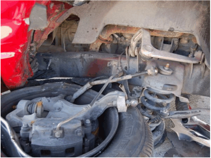
Figure 53. Undercarriage Damage, Test No. TCBT-1
