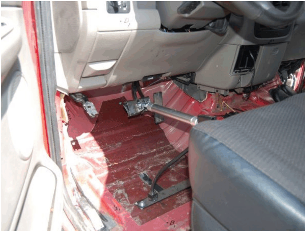
Figure 54. Occupant Compartment Deformation, Test No. TCBT-1
