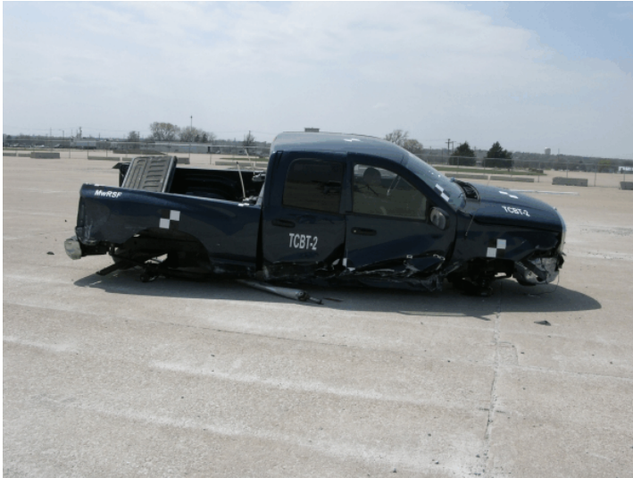
Figure 65. Vehicle Damage, Test No. TCBT-2
