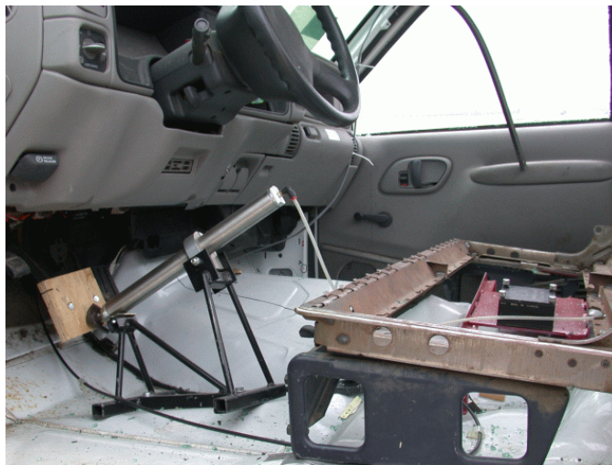
Figure 33. Windshield and Occupant Compartment Damage, Test MOBR-1
