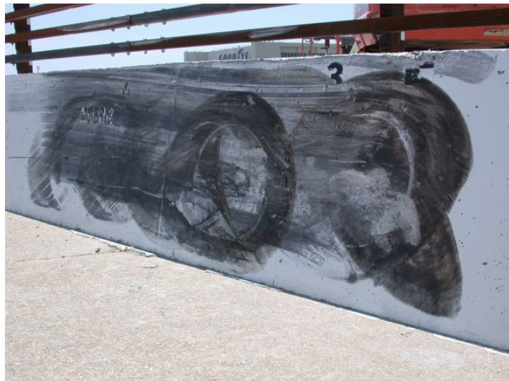
Figure 53. System Damage, Test MOBR-2
