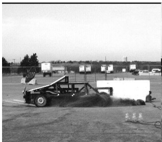
Figure 8. Sequential Photographs – 0 degree orientation, Bogie Test MN1C-0
