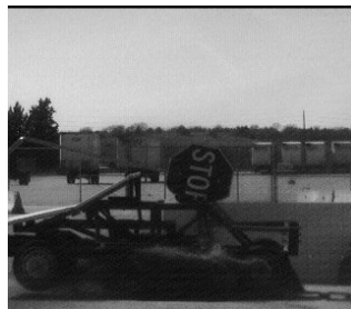
Figure 57. Sequential Photographs – 90 degree orientation, Bogie Test MN8A-90
