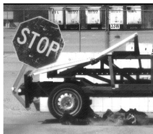
Figure 9. Sequential Photographs – 90 degree orientation, Bogie Test MN1C-90
