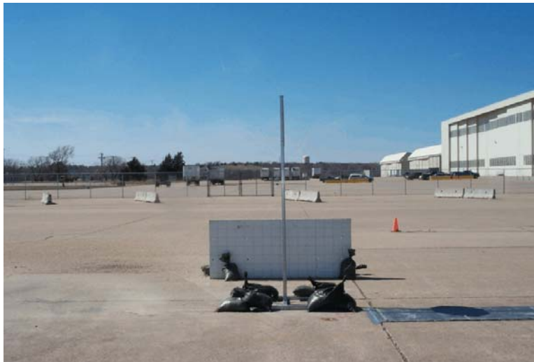
Figure 51. Stop Sign System with 7' Mounting Height, Bogie Tests MN8A-0 and MN8A-90
