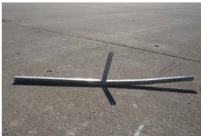
Figure 38. 48" x 48" Diamond Panel Work Zone Sign System with 5' Mounting Height Damage, Bogie Test MN6A-0 (0 degrees)
