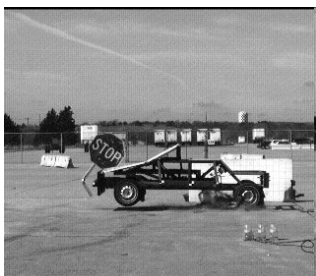
Figure 9. Sequential Photographs – 90 degree orientation, Bogie Test MN1C-90
