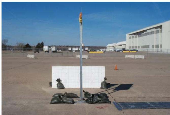
Figure 34. 48" x 48" Diamond Panel Work Zone Sign System with 5' Mounting Height, Bogie Tests MN6A-0 and MN6A-90
