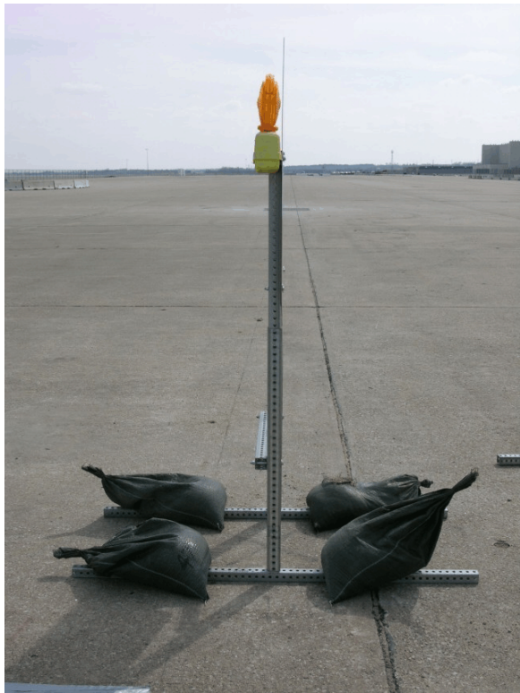
Figure 27. 36" x 36" Diamond Work Zone Sign System, Bogie Tests MN5C-90-2
