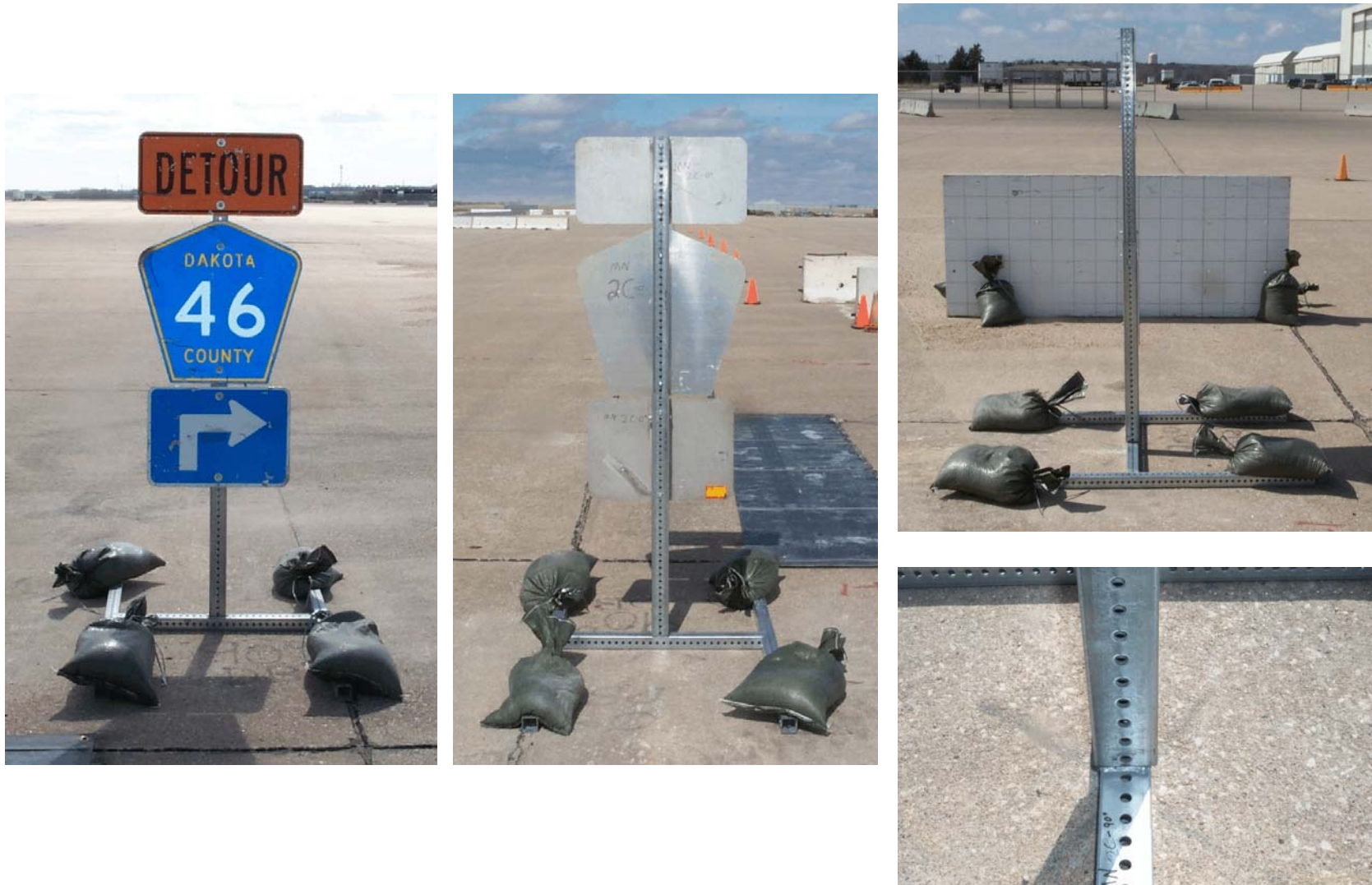
Figure 10. Route Marker Assembly System, Bogie Tests MN2C-0 and MN2C-90
