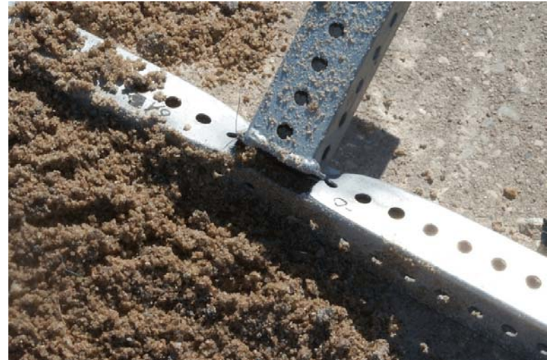
Figure 54. Stop Sign System with 7' Mounting Height Damage, Bogie Test MN8A-0 (0 degrees)
