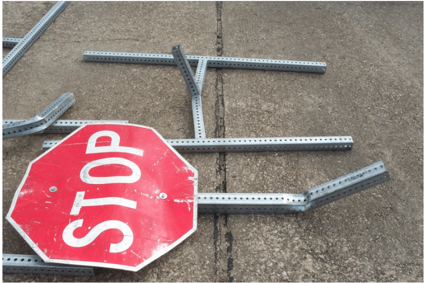
Figure 6. Stop Sign System Damage, Bogie Test MN1C-0 (0 degrees)
