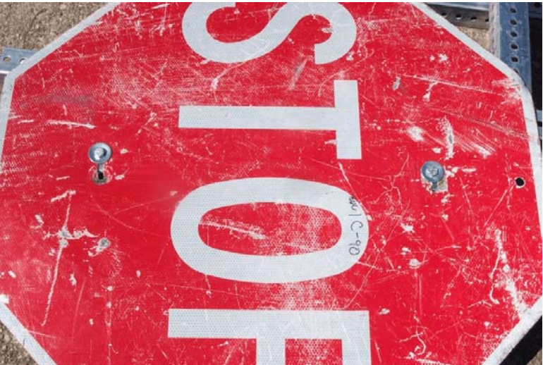
Figure 7. Stop Sign System Damage, Bogie Test MN1C-90 (90 degrees)
