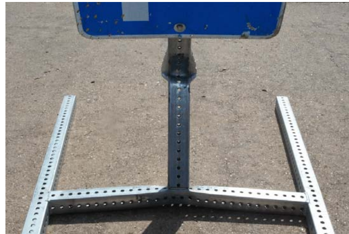
Figure 13. Route Marker Assembly System Damage, Bogie Test MN2C-0 (0 degrees)
