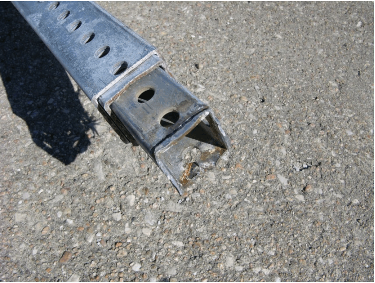
Figure 21. Work Zone Speed Limit Sign System Damage, Bogie Test MN3B-0-2 (0 degrees)
