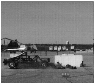
Figure 41. Sequential Photographs – 90 degree orientation, Bogie Test MN6A-90
