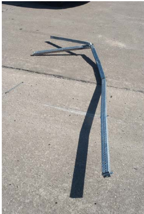
Figure 39. 48" x 48" Diamond Panel Work Zone Sign System with 5' Mounting Height Damage, Bogie Test MN6A-90 (90 degrees)
