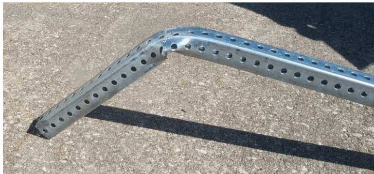
Figure 54. Stop Sign System with 7' Mounting Height Damage, Bogie Test MN8A-0 (0 degrees)
