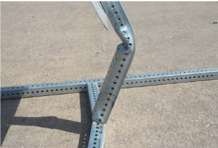
Figure 13. Route Marker Assembly System Damage, Bogie Test MN2C-0 (0 degrees)
