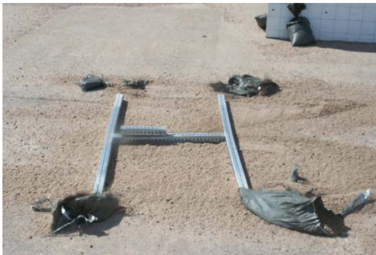
Figure 14. Route Marker Assembly System Damage, Bogie Test MN2C-90 (90 degrees)
