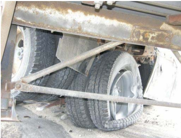
Figure 90. Vehicle Damage to Front Tandems, Test TL5CMB-2
