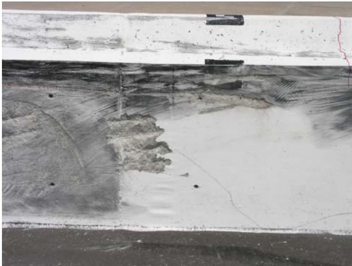
Figure 80. Barrier Damage, Gouges 9.1 - 11.0 m (30 - 36 ft) from Upstream End, Test TL5CMB-2
