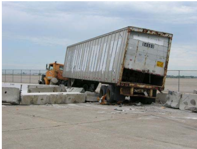
Figure 85. Vehicle Damage, Test, TL5CMB-2
