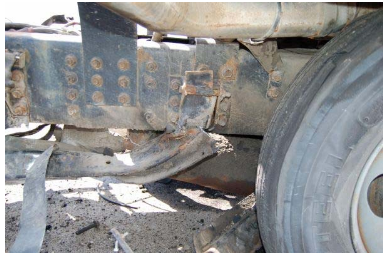
Figure 88. Right Side Tractor Damage, Test TL5CMB-2
