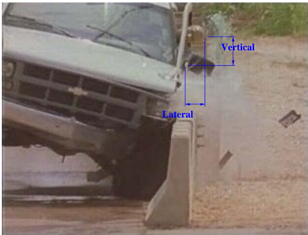
Figure 8. Lateral and Vertical Measurements from the Bottom of the Window
