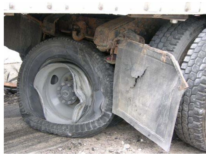
Figure 90. Vehicle Damage to Front Tandems, Test TL5CMB-2
