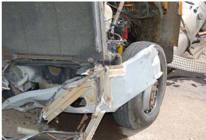
Figure 86. Front Bumper Damage, Test TL5CMB-2
