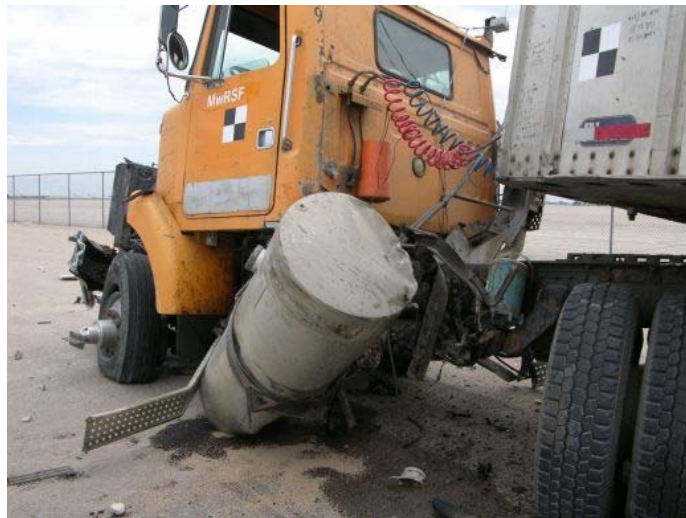
Figure 89. Left Side Tractor Damage, Test TL5CMB-2 198
