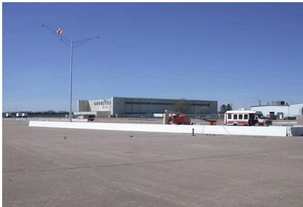
Figure 10. Luminaire Pole Attach to Single-Slope Concrete Barrier, Test Nos. ZOI-1 and ZOI-2
