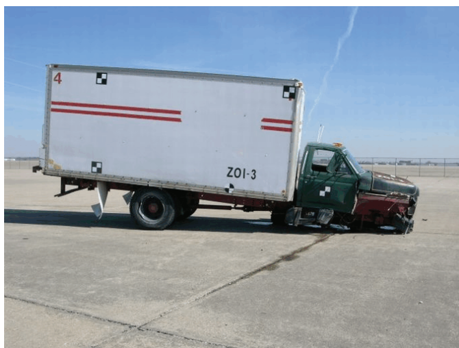
Figure 73. Vehicle Damage, Test No. Z01-3
