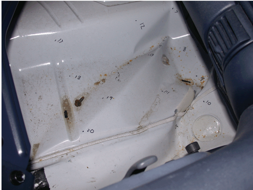
Figure 55. Occupant Compartment Deformation, Test No. ZOI-2
