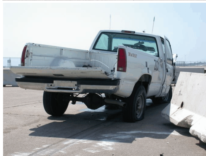
Figure 52. Vehicle Damage, Test No. ZOI-2
