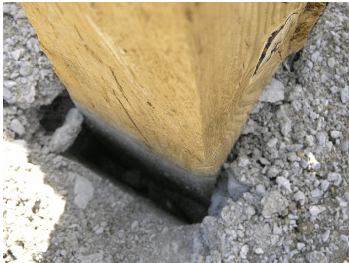
Figure 61. Soil Failure, Test SR-5
