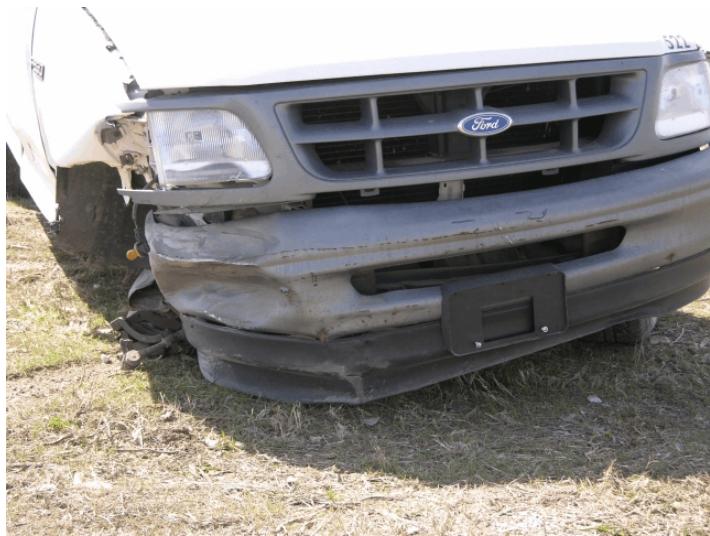
Figure 63. Vehicle Damage, Test SR-5
