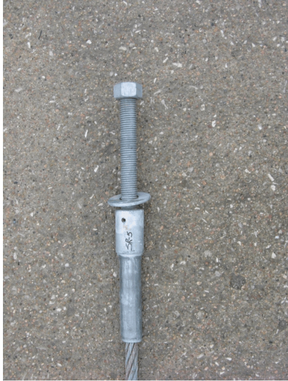
Figure 56. Nose Cable Damage, Test SR-5
