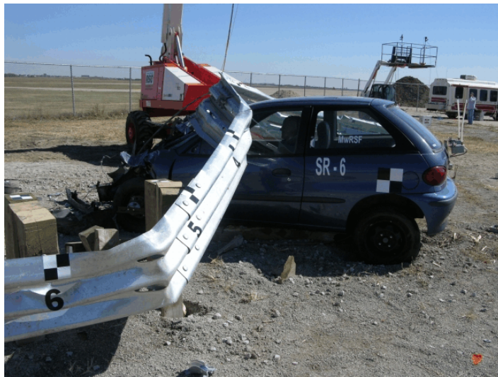
Figure 88. System Damage, Test SR-6
