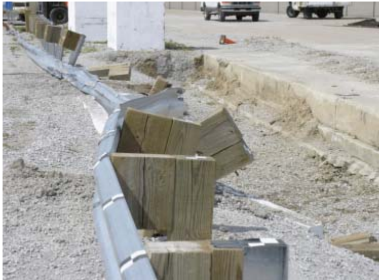
Figure 59. System Overall Damage, Test No. LSC-2
