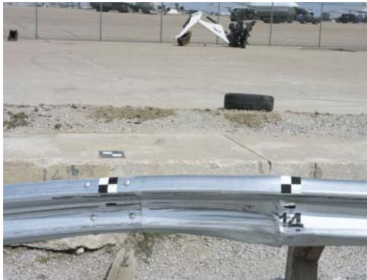
Figure 62. System Rail Damage, Test No. LSC-2
