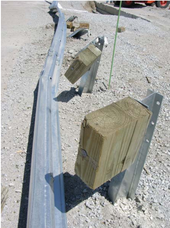
Figure 34. System Post Damage, Test No. LSC-1
