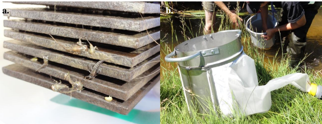
Figure 4. Photos of a) Hester-Dendy sampler colonized by aquatic invertebrates and b) Hess sampler.
